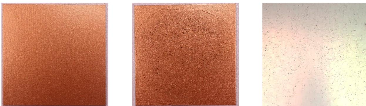
**Figure 5.** Initially clean PVDF sample (left), PVDF sample with wet-applied 4000 mgm<sup>-2</sup> of deposit (middle), and observed natural deposit on the building (right).
