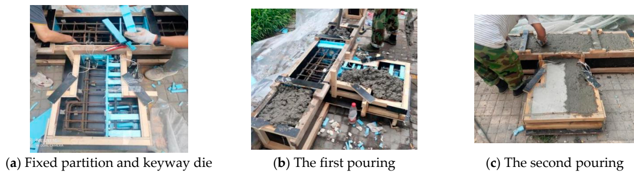
Figure 2. Key production process of specimens.
