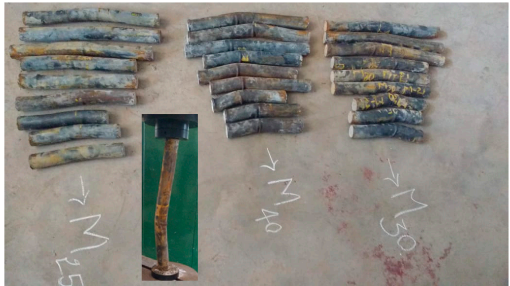
Figure 5. Failure modes of SCCFSTs.
