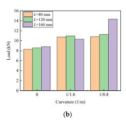
Figure 6. Effect of circular arc curvature on load capacity: (a) one-layer CFRP; (b) two-layer CFRP.
