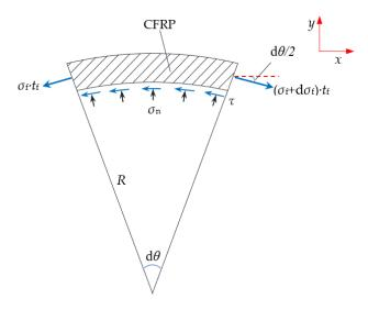
**Figure 7.** Load condition per unit width of an infinitesimal element of CFRP with a convex-circular arc interface.
