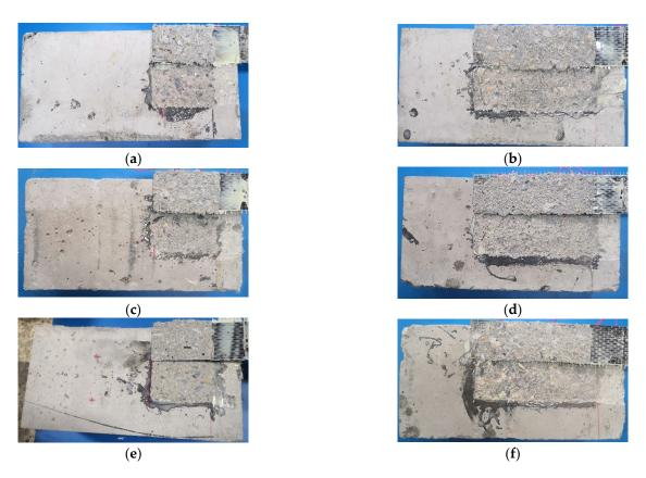
**Figure 4.** CFRP debonding failure of the specimens: (a) K1L80P1; (b) K1L160P1; (c) K2L80P1; (d) K2L160P1; (e) K1L80P2; (f) K3L160P2.
