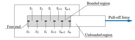
Figure 9. Schematic diagram of strain and bond stress.
