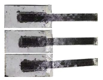
Figure 2. View of some bonding specimens.
