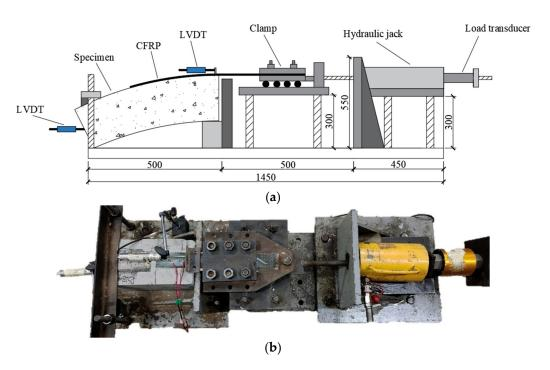
Figure 3. View of single shear test: (a) schematic diagram (K3 series specimen); (b) test picture.
