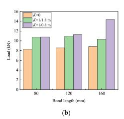
Figure 5. Effect of bond length on load capacity: (a) one-layer CFRP; (b) two-layer CFRP.
