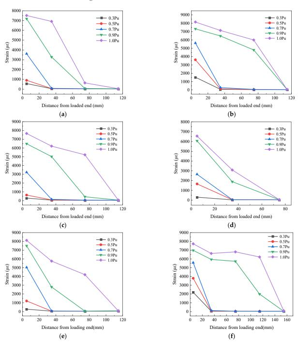
**Figure 8.** CFRP strains along its length: (a) K1L120P2; (b) K2L120P2; (c) K3L120P2; (d) K3L80P1; (e) K3L120P1; (f) K3L160P1.
