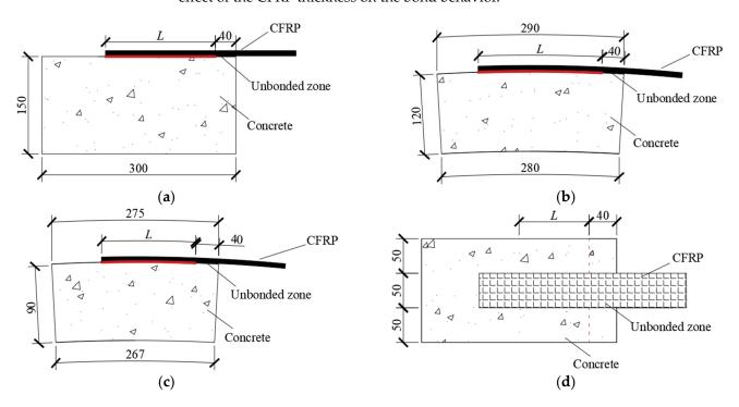
**Figure 1.** Schematic diagram of bond specimens. (a) side view of K1 series; (b) side view of K2 series; (c) side view of K3 series; (d) plan view of all series.
