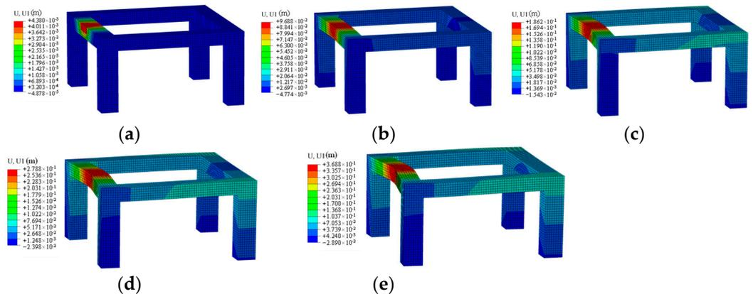
Figure 4. Contours of the lateral displacement of the transmission tower foundation under different impact durations: (a) initial impact time; (b) 10 ms; (c) 20 ms; (d) 30 ms; (e) 40 ms.
