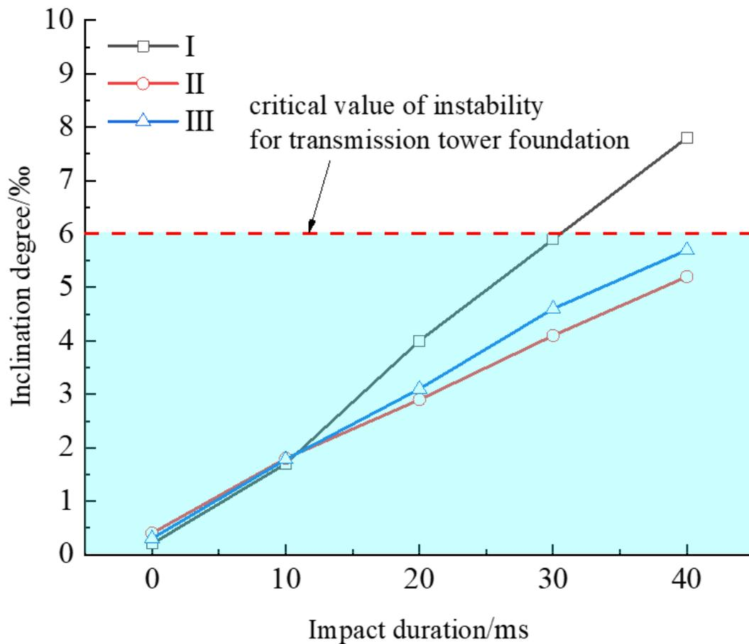
**Figure 8.** Inclination degrees of the transmission tower foundation under different impactor shapes.
