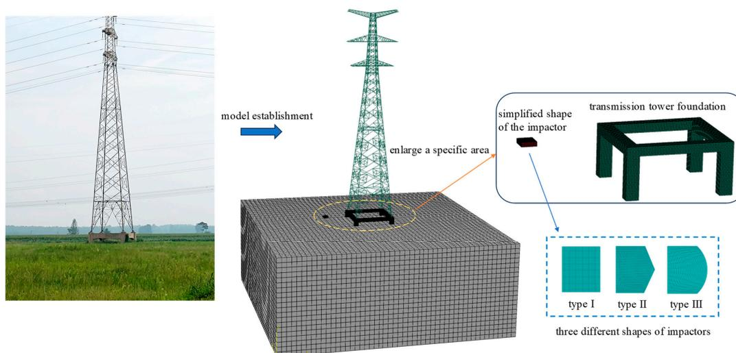
**Figure 1.** Schematic diagram of the numerical model of the transmission tower foundation.
