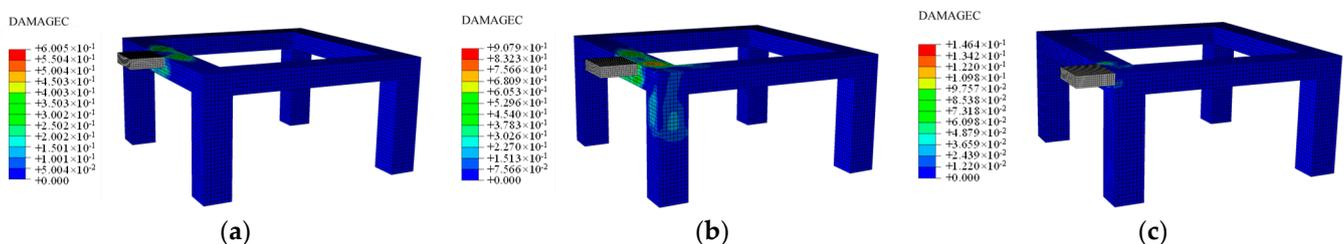
**Figure 9.** Compression damage contours of the type I impactor at different locations at the initial impact time: (a) impact mid-span position; (b) impact quarter-span position; (c) impact edge position.
