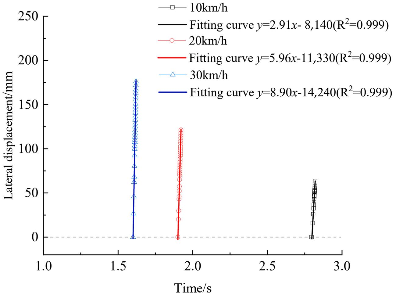
Figure 3. Lateral displacement time history curves of unit node A under different impact velocities.
