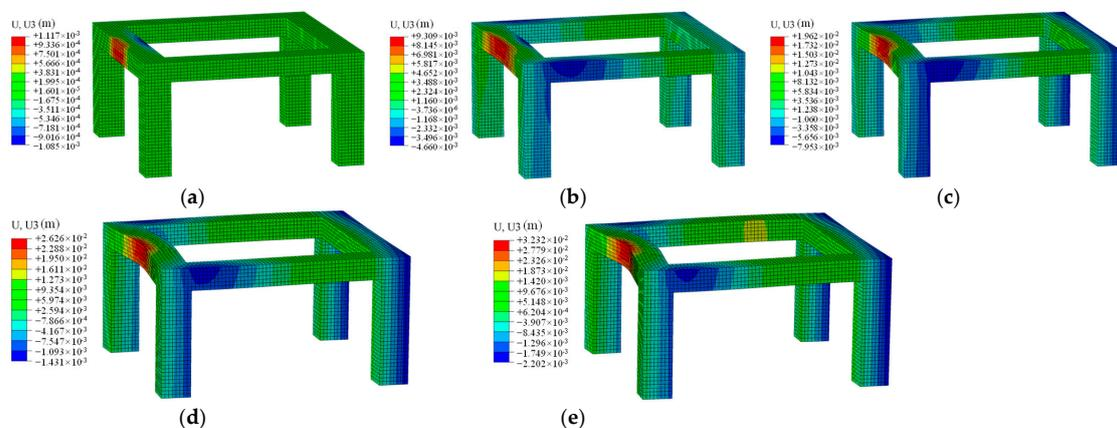
**Figure 6.** Vertical displacement contours of the transmission tower foundation under different impact durations: (a) initial impact time; (b) 10 ms; (c) 20 ms; (d) 30 ms; (e) 40 ms.
