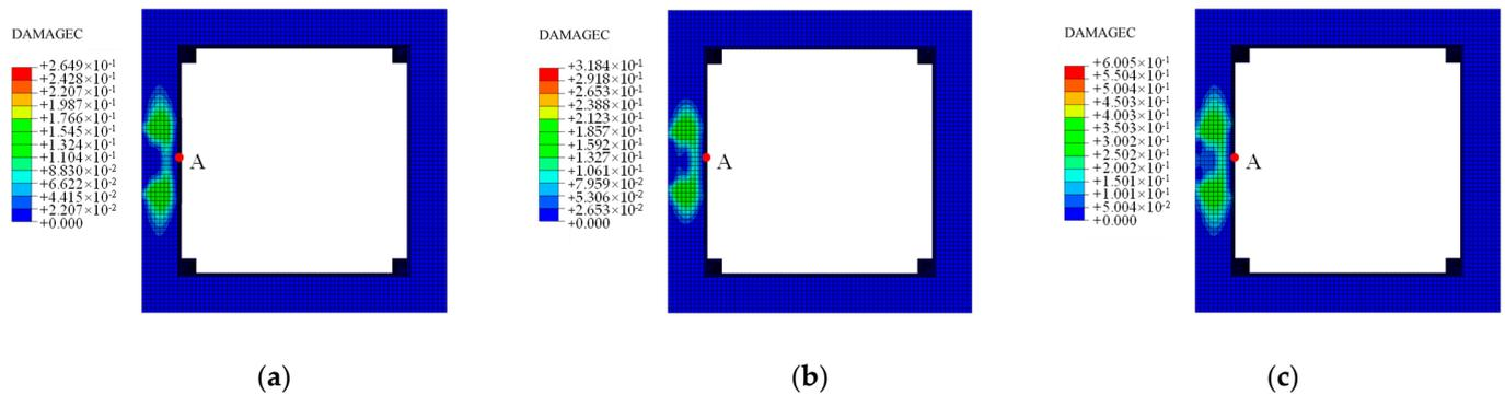
**Figure 2.** Compression damage contours of the transmission tower foundation at initial impact time under different impact velocities: (a)  $v = 10$  km/h; (b)  $v = 20$  km/h; (c)  $v = 30$  km/h.
