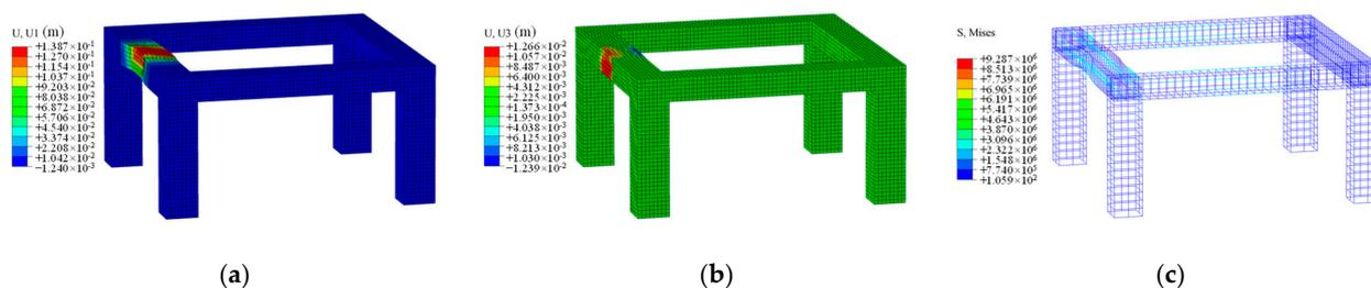
**Figure 12.** Contours of the lateral displacement, vertical displacement, and rebar cage stress of reinforced transmission tower foundation: (a) lateral displacement; (b) vertical displacement; (c) steel skeleton stress contour.
