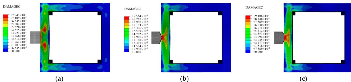
**Figure 7.** Contours of the compression damages of the transmission tower foundation under different impactor shapes: (a) type I; (b) type II; (c) type III.
