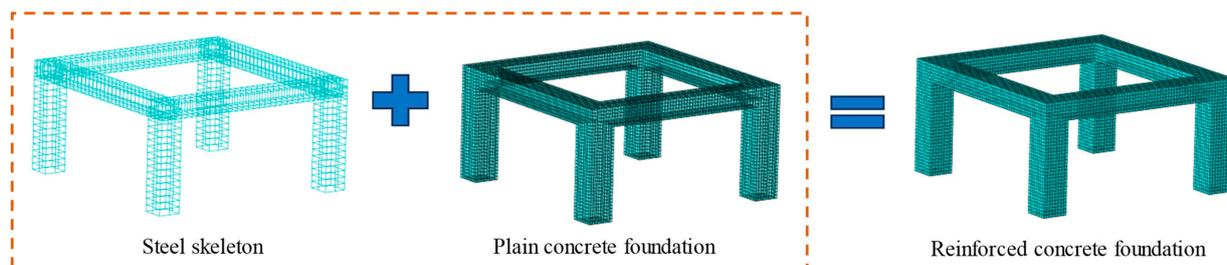
**Figure 11.** Schematic diagram of the numerical model of the reinforced transmission tower foundation.
