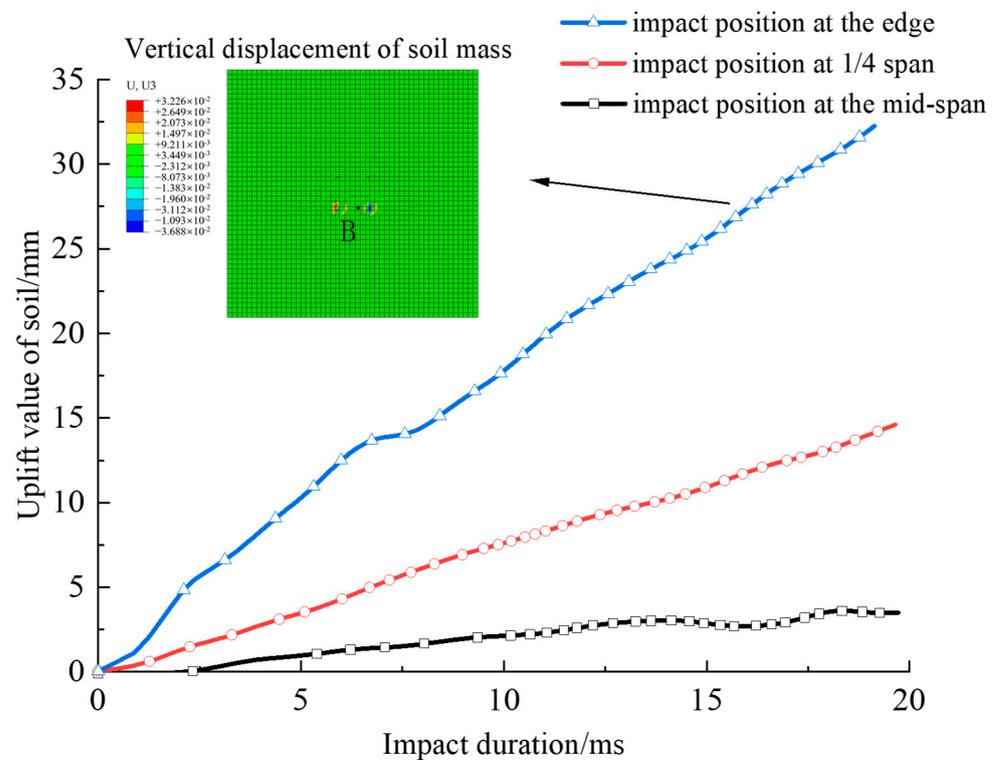
**Figure 10.** Variation curves of the uplift value of unit node B at the left front corner of the transmission tower foundation.
