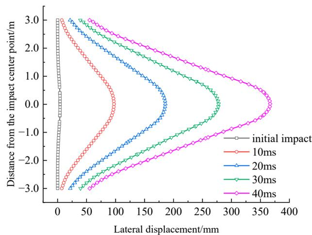
**Figure 5.** Lateral displacement values of individual points along the longitudinal center line of the impact beam.
