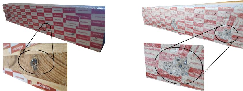
The failure is announced by an opening of the gap between concrete and CLT
