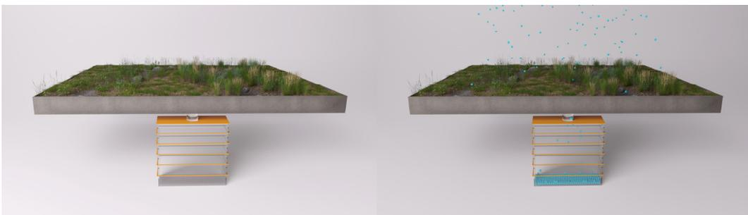
**Figure 8.** Visualization of the intensive green roof before and after the simulation. The total accumulated amount of runoff water to the stormwater tank is  $0.25 \text{ m}^3$ .
