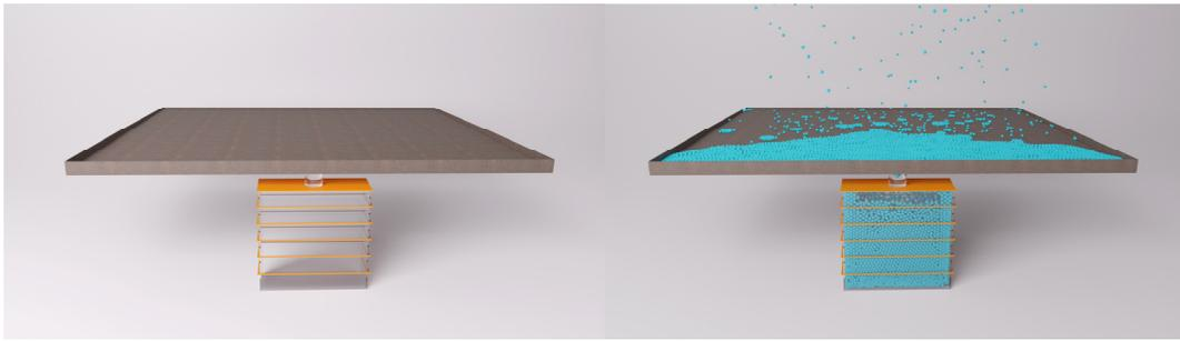
**Figure 6.** Visualization of the bitumen roof before and after the simulation. The total accumulated amount of runoff water to the stormwater tank is  $8.5 \text{ m}^3$ .
