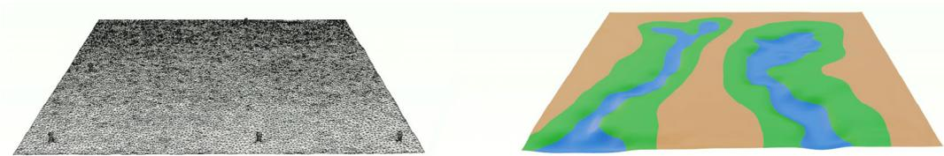
**Figure 2.** A rapid method for visualization by changing the colour scheme and topography of the mesh model. On the left side is the original 3D mesh of the test site based on photogrammetry. On the right side is the illustration of a surface water reservoir by altering the surface topography of the mesh. Further, the colour scheme has been enhanced to highlight the wider adoption of a green roof.
