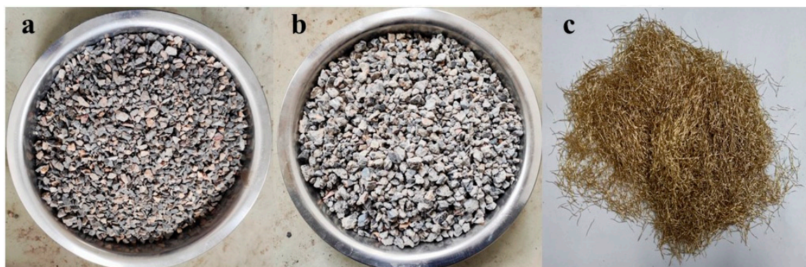
Figure 1. Apparent morphologies of (a) NAs; (b) RAs; (c) SFs.
