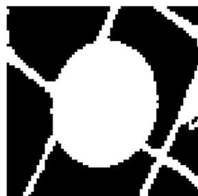
**Figure 16.** Example of Otsu at ellipse target 1.
