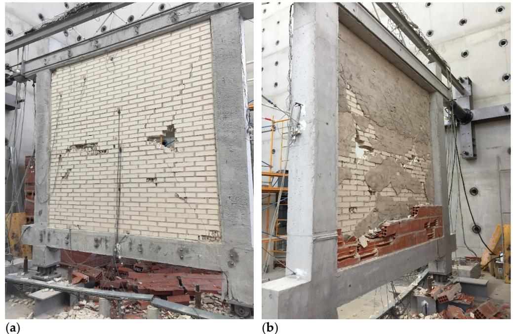
**Figure 19.** Damages in the pre-existing cladding at the end of the test: (a) front view of the sample. State of the facing brick sheet after removing the ventilated façade sheet; and (b) rear view of the sample. State of the interior facing brick sheet.
