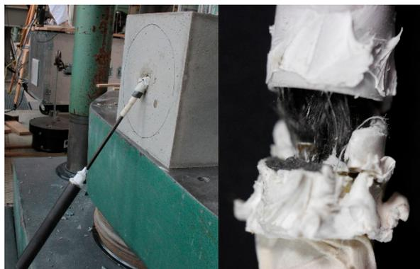
**Figure 6.** Failed carbon rebar 5 (photo: A. Schumann).
