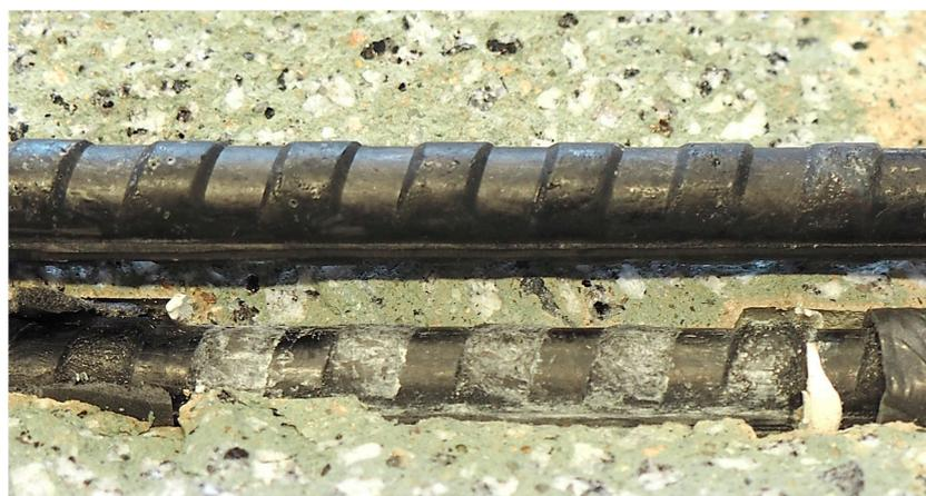
**Figure 1.** Carbon rebar with destroyed lugs of the rebar (photo: A. Schumann).
