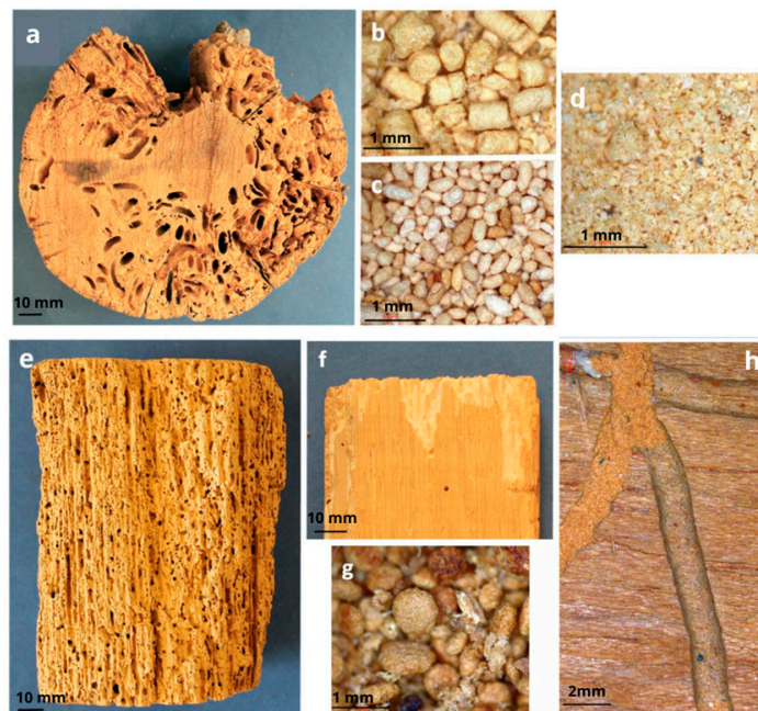
Figure 3. Galleries, exit holes, and dust excrements of widespread wood-deteriorating beetles in Europe: (a) oval galleries bored by Hylotrupes bajulus ( Cerambycidae ) in a cross section of a utility pole; (b) cylindrical dust excrements typical of Cerambycidae ; (c) dust excrements of Anobium punctatum ( Anobiidae ); (d) amorphous dust excrements characteristic of Lyctinae ( Bostrichidae ); (e) wood heavily attacked by Anobiidae members; (f) skirting board attacked by Lyctinae ( Bostrichidae ) members; (g) dust excrements of Xestobium rufovillosum ( Anobiidae ); (h) a larval gallery partially filled with soft-to-the-touch dust excrements, bored by Lyctinae ( Bostrichidae ) members. (Readapted with permission from Ref. [21]. 2023, Martín J.A. and López R.).
