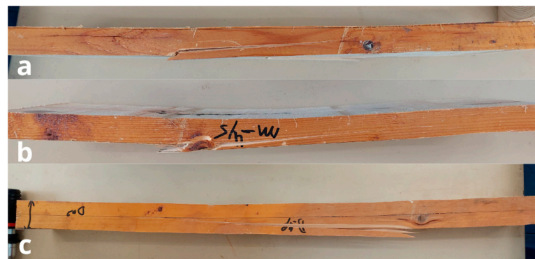
Figure 17. Tested specimens: (a) wood failure type of single laminates; (b) knot presence in a tested 1.3.3 specimen of SS 1.3; (c) knot presence in a tested double laminate.
