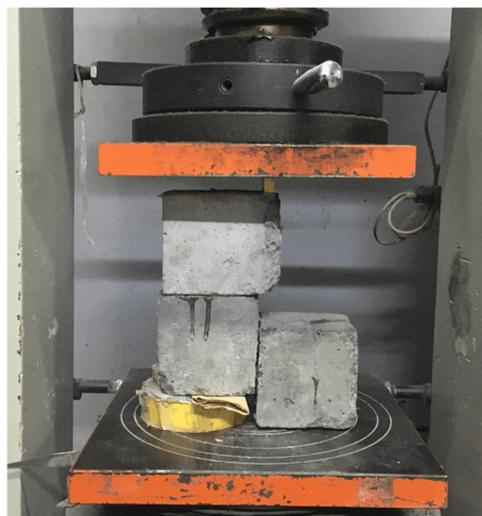
**Figure 9.** Straight shear test.
