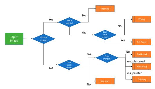
Figure 9. The logical map for identifying the different states of drywall installation.
