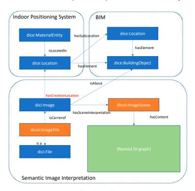
**Figure 10.** Data mapping of the drywall operation DTC.
