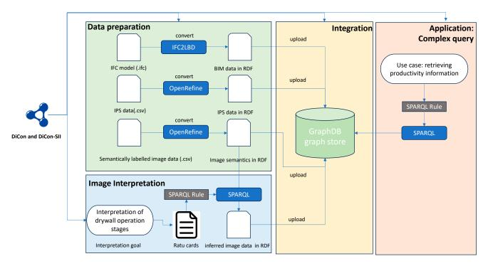
Figure 7. The implementation architecture of the case study.
