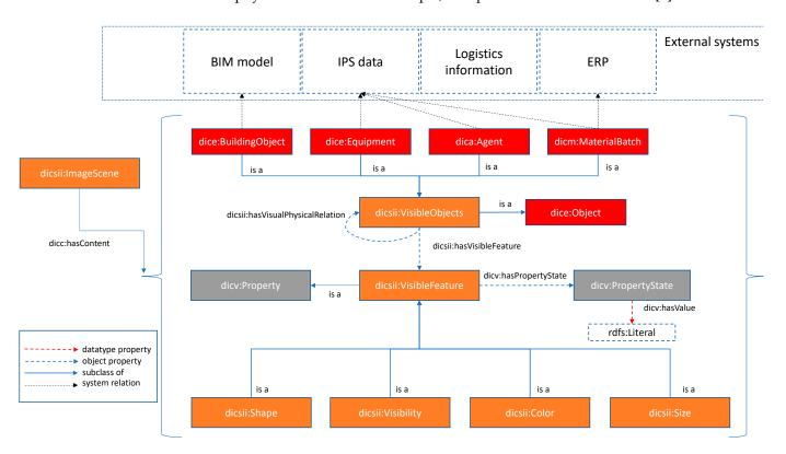
Figure 6. The detailed ontological model for describing construction image contents.
