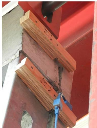
**Figure 17.** Relative displacement of integrated concrete beam to shell at failure.
