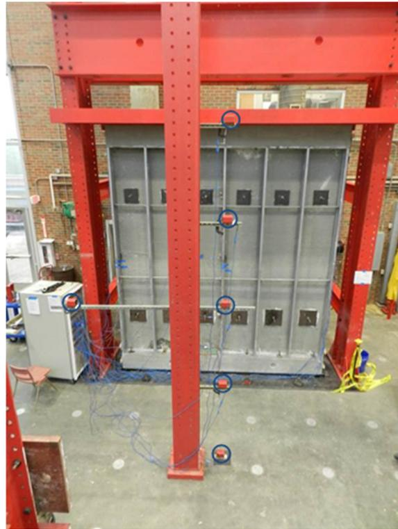
**Figure 6.** String potentiometer positions.
