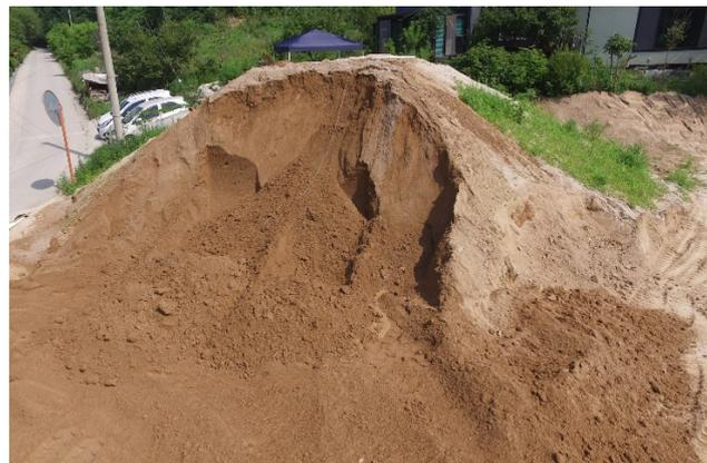
**Figure 4.** Field model slope failure.
