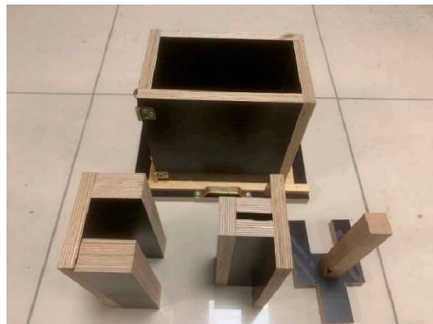
**Figure 5.** Main plywood mould, back piece, front piece, and wooden hand.
