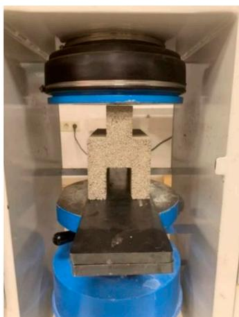
**Figure 8.** Standard interlocking concrete block in the compression test machine.
