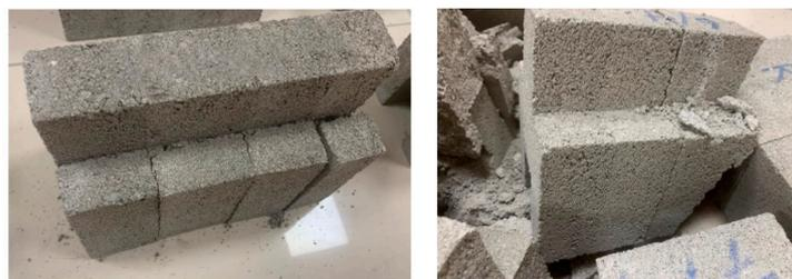
**Figure 16.** Vertical lines of cracks after loading axial force.
