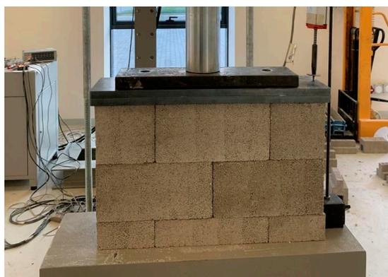
**Figure 9.** ICB wallette specimen test setup.
