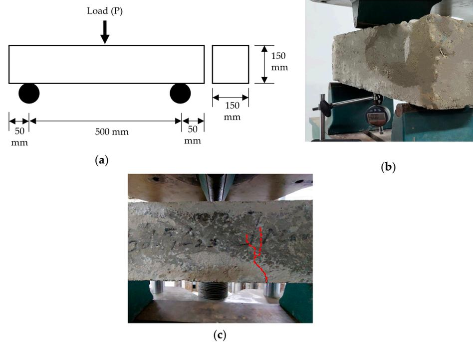
**Figure 5.** (a) Dimensions of the concrete beam specimens, (b) test setup for the flexural strength of concrete using beam specimens, and (c) a beam specimen after failure.
