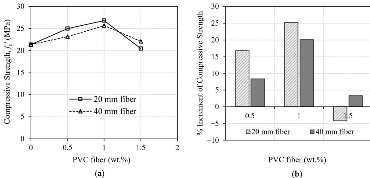
**Figure 8.** Effects of PVC fiber content and length on the (a) compressive strength and (b) % increment of compressive strength of concrete.
