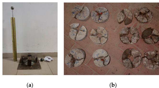
**Figure 6.** (a) Test apparatus for impact test and (b) failure of the specimens after impact testing.
