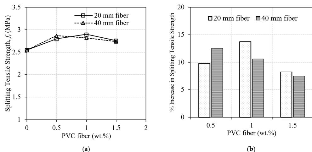
**Figure 10.** Effects of PVC fiber content and length on the (a) splitting tensile strength and (b) % increment of splitting tensile strength of concrete.
