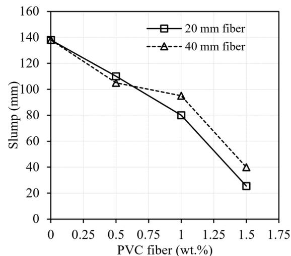
**Figure 7.** Effects of PVC fiber content and length on the workability of concrete.
