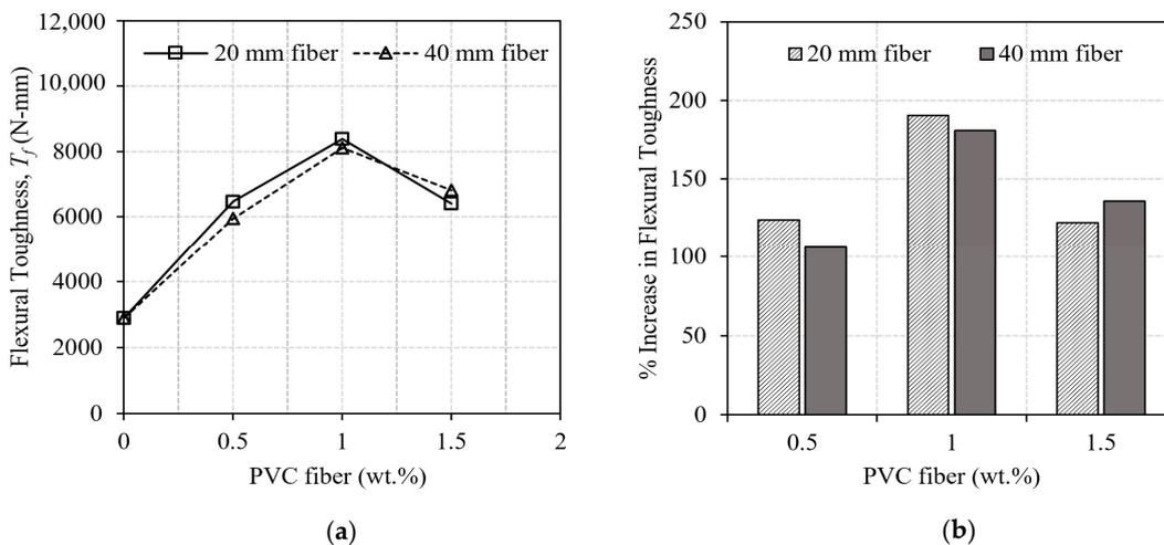
Figure 14. Effects of PVC fiber content and length on the (a) flexural toughness and (b) % increase in flexural toughness of concrete.
