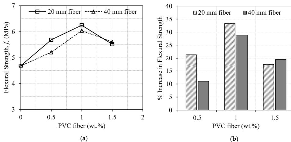
Figure 13. Effects of PVC fiber content and length on the (a) flexural strength and (b) % increase in flexural strength of concrete.
