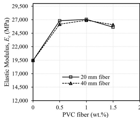
**Figure 9.** Effects of PVC fiber content and length on the static elastic modulus of concrete.
