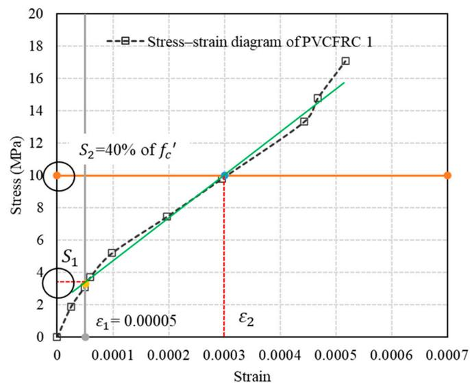
**Figure 4.** Stress–strain diagram of a concrete (PVCFRC 1) to determine its static elastic modulus.
