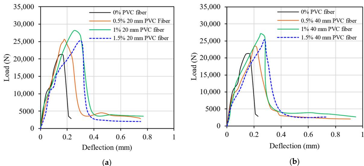
**Figure 12.** Load-deflection behavior of the concretes with (a) 20 mm and (b) 40 mm long PVC fibers.
