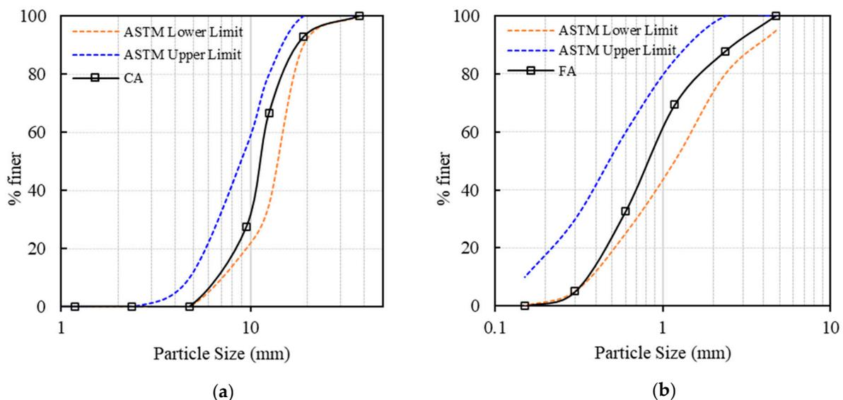
**Figure 1.** Particle size distribution of (a) coarse aggregate and (b) fine aggregate.
