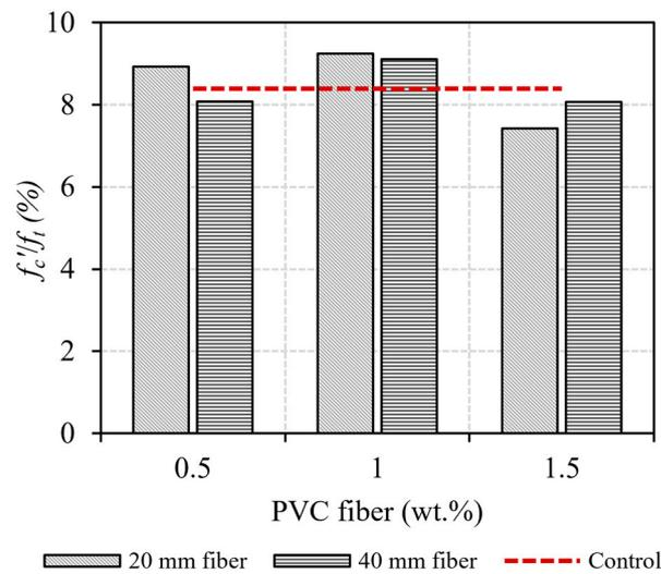
**Figure 11.** Influence of PVC fiber content on the percentage of compressive to tensile strengths of concrete.
