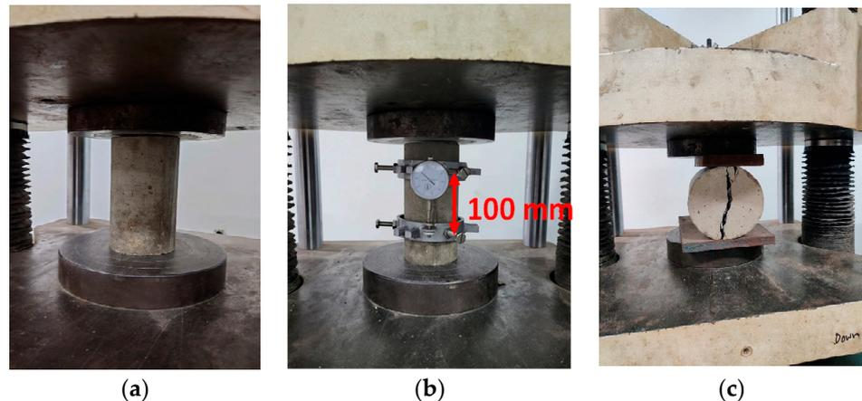
**Figure 3.** Tests for the (a) compressive strength, (b) static elastic modulus, and (c) splitting tensile strength of concrete.
