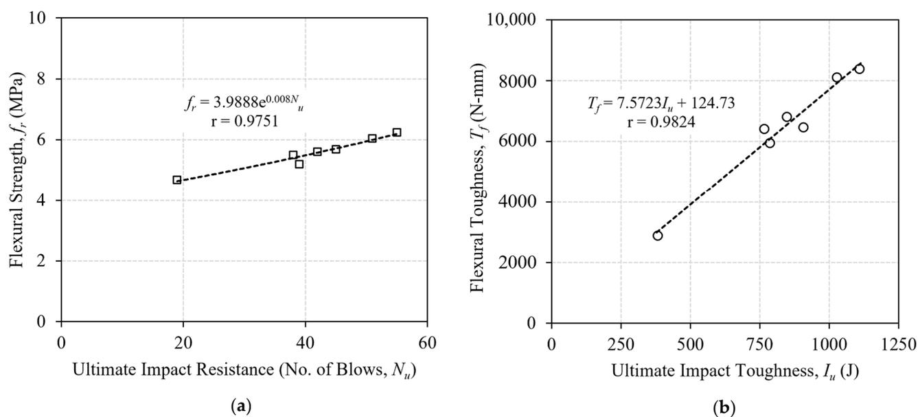
**Figure 17.** Correlations of the (a) flexural strength and ultimate impact resistance, and (b) flexural toughness and ultimate impact toughness of concrete.
