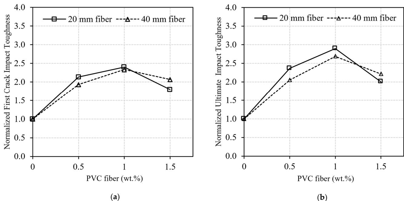
**Figure 15.** Normalized (a) first crack impact toughness and (b) ultimate impact toughness of concrete.
