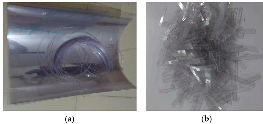
**Figure 2.** Processing of plastic fibers (a) PVC sheets and (b) PVC fibers after cutting.
