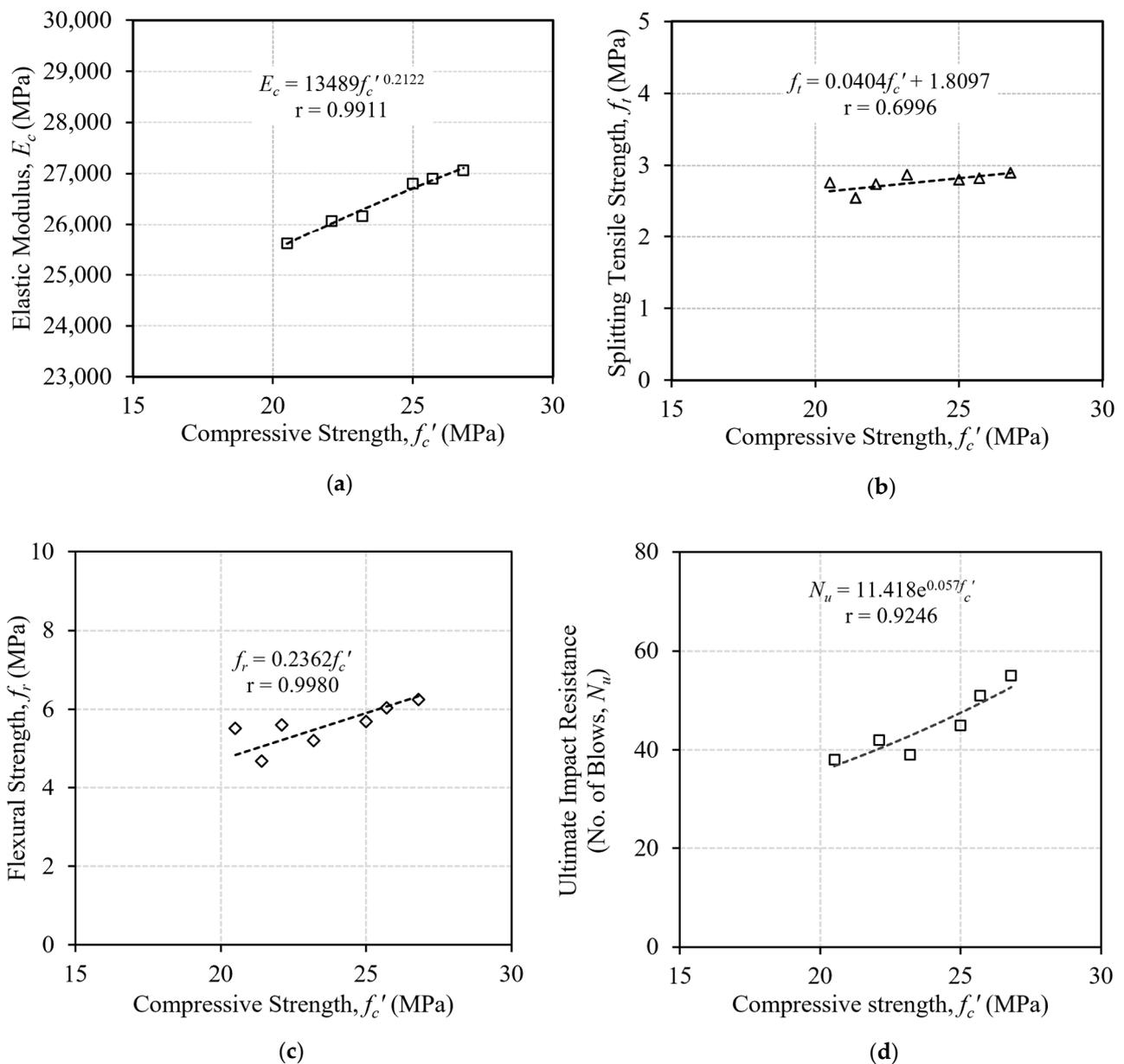
**Figure 16.** Correlations of the compressive strength of concrete with its (a) elastic modulus, (b) splitting tensile strength, (c) flexural strength, and (d) ultimate impact resistance.
