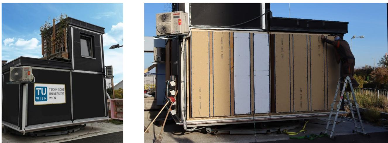
Figure 1. Outdoor test rig for the examination of exterior walls in Vienna, Austria.
