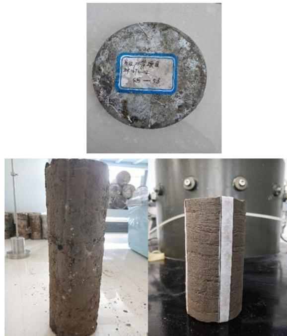
**Figure 2.** Soft clay sample with intercalated sand. (Taken from Binjiang Waterfront Project, No. zk167-02, 515-518).
