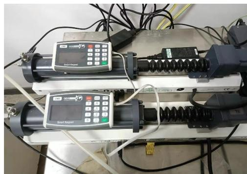
(a) Dynamic confining pressure and servo motor (b) Pressure control system diagram machine
