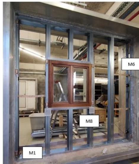
**Figure 8.** Test specimen structure from SMARTLSF project with integrated sensors (external view).
