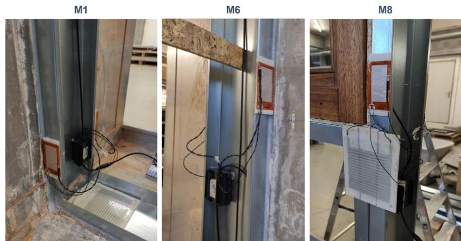
**Figure 9.** Detailed images of the integration of three modules (identified as M1, M6, and M8 in Figure 8) in distinct positions.
