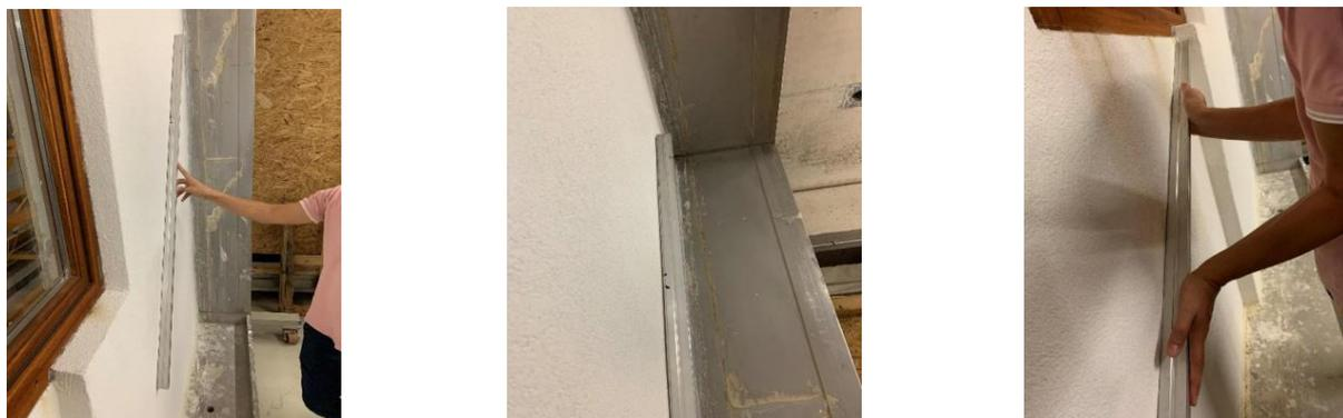
**Figure 24.** Images of the visual inspection performed after the hygrothermal cycles.
