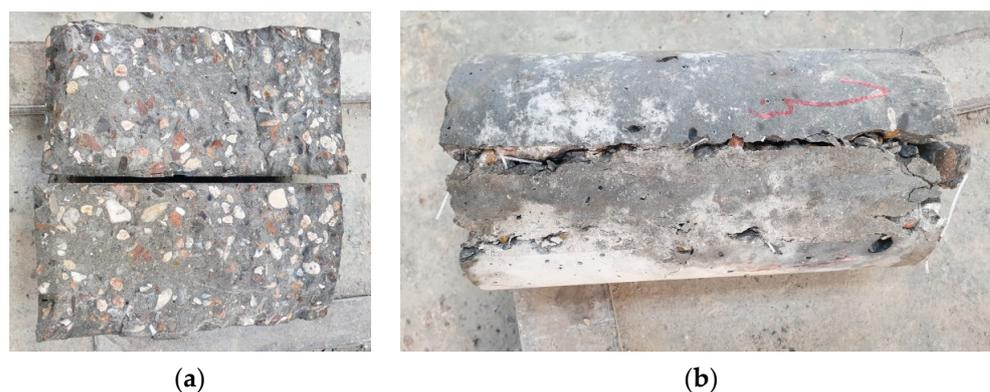
**Figure 8.** Splitting test for concrete specimens: (a) without fiber; (b) with fiber.
