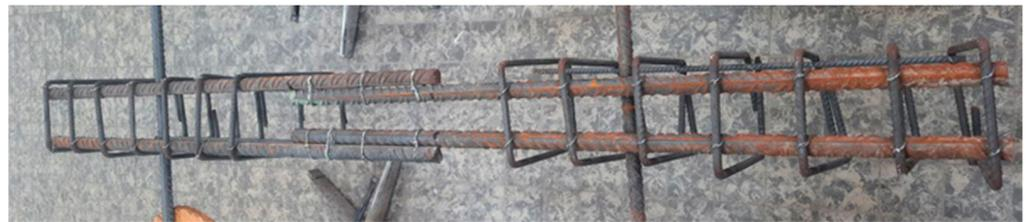
Figure 4. Lap splices reinforcement of beam specimen.
