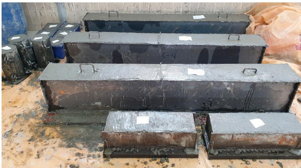
**Figure 6.** Concrete test specimens.
