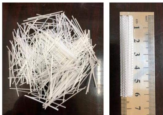
**Figure 5.** Macro polyolefin fibers.
