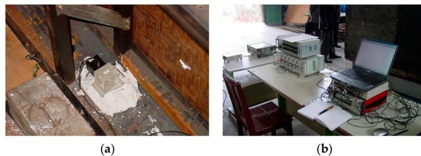
**Figure 2.** Data acquisition instruments: (a) accelerometer; (b) signal acquisition device.
