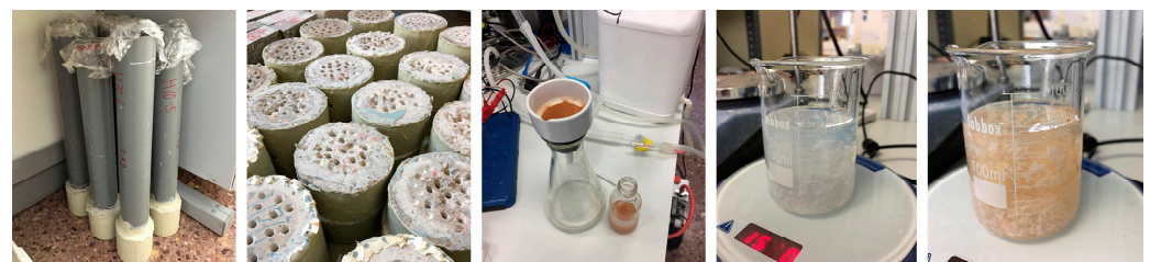
Figure 4. Setup for the chloride diffusion test and the chloride analysis.
