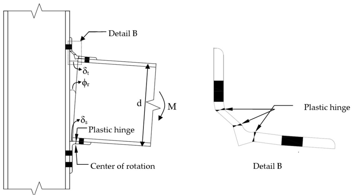
Figure 6. Deformation shape of a TSAC.
