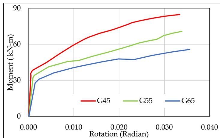
**Figure 15.** Effect of bolt gage distance.
