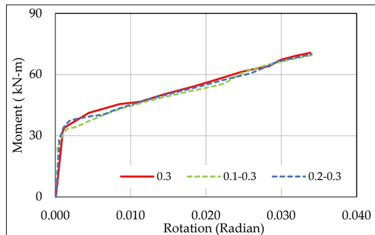
Figure 12. Effect of the different friction coefficients between the beam, column, and angles.
