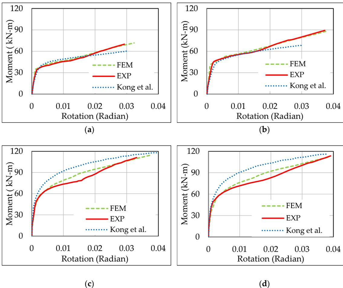
**Figure 7.** Comparisons of the M– $\theta$  curves: (a) T10–S12, (b) T10–S15, (c) T13–S12, (d) T13–S15 [8,17].
