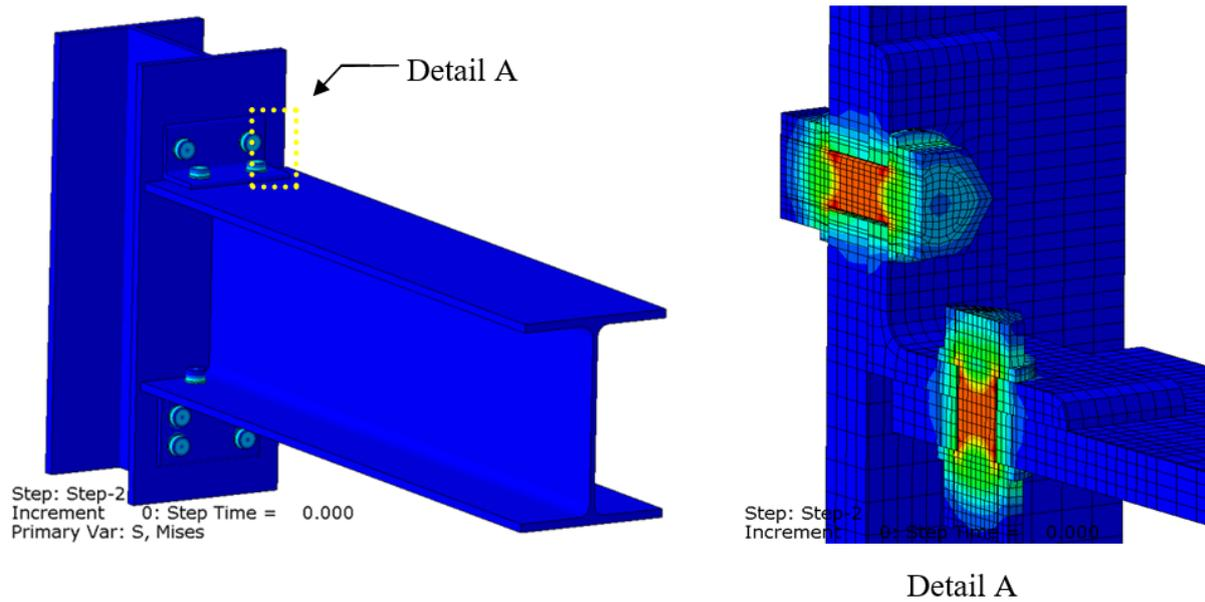
Figure 5. The pre-stress transfer to the flange and the angle.
