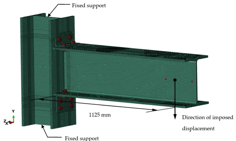
**Figure 3.** Boundary conditions and mesh pattern of FE model.
