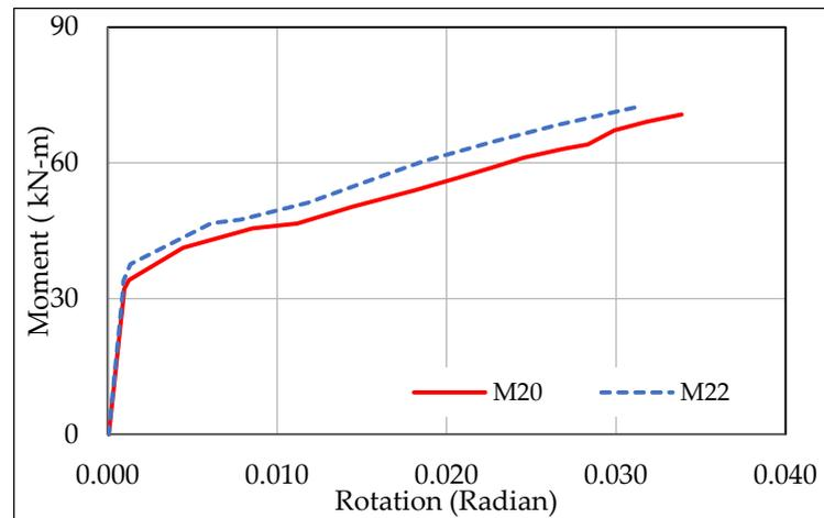
**Figure 14.** Effect of bolt diameter.
