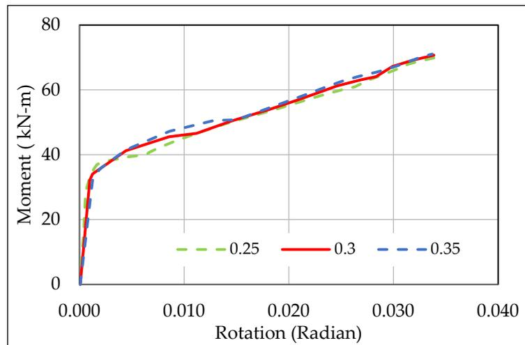
Figure 11. Effect of different friction coefficient between all the contact surfaces.
