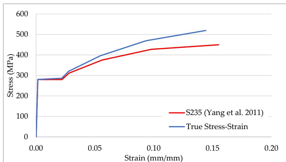
**Figure 2.** Engineered and true stress–strain curves of S235 steel material [16].
