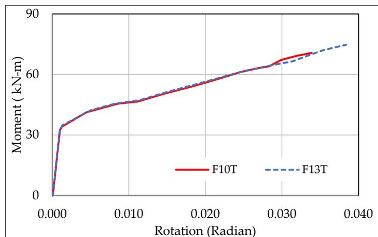
Figure 13. Effect of bolt strength.
