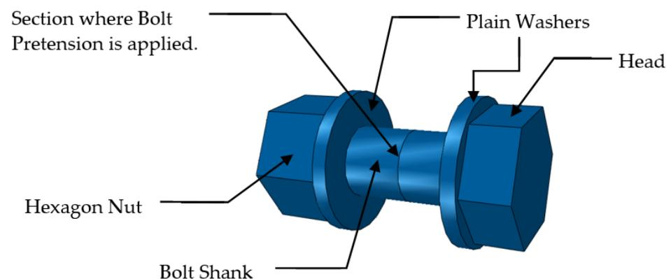
**Figure 4.** Details of the bolt used in FE model.
