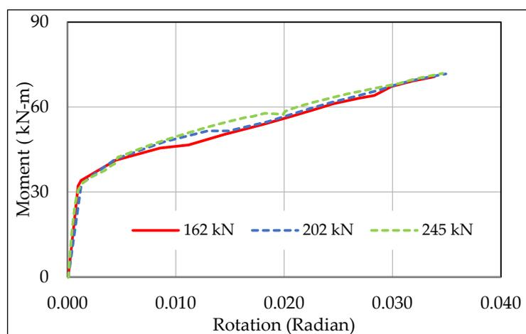
Figure 10. Effect of the bolt pretension force.
