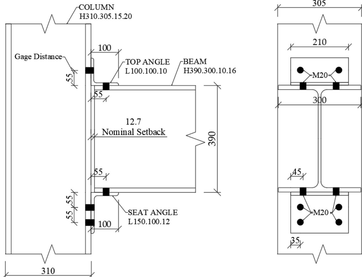
Figure 1. Geometry of T10-S12 connection.
