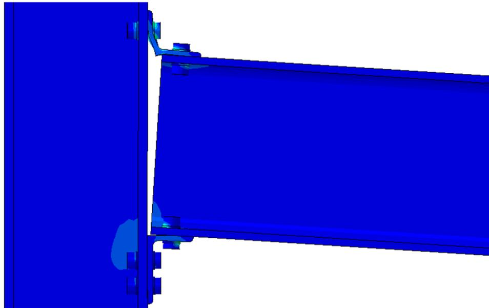
Figure 8. Deformed shape of T10-S15 angle connection.
