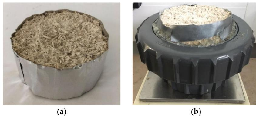
**Figure 5.** Hygric property characterization: (a) sample for the MBV test; (b) set-up for the water vapor permeability test.
