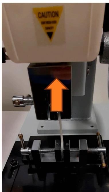
**Figure 1.** A 3D-printed dog-bone sample under tensile test.
