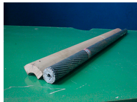
Figure 3. Test transmission conductor.
