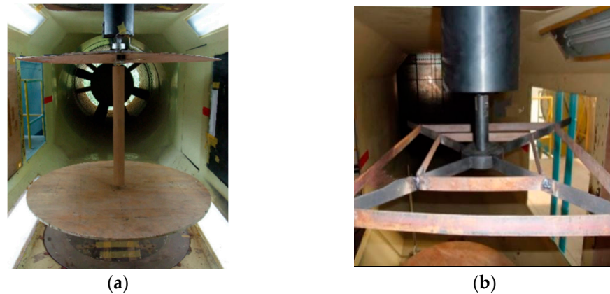
Figure 4. Aerodynamic force measurement test system for iced conductor: (a) wind tunnel test; (b) test model support device.
