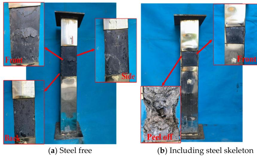
Figure 11. Failure modes of typical specimens.
