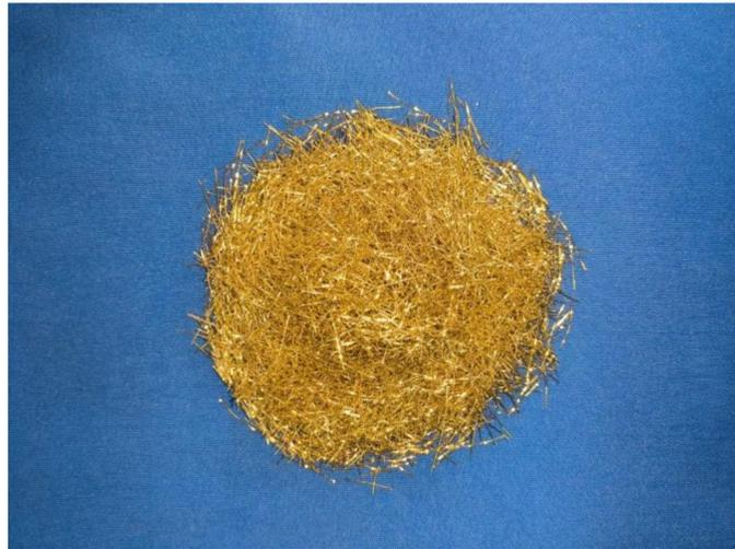
**Figure 2.** Steel fiber samples.
