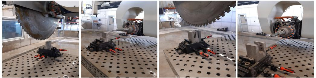
**Figure 23.** F8: milling process of both couples; left-pare: duration: 8 min, speed: 50%, Ra: 500 (rad/min); right-pare: duration: 15 min, speed: 50%, Ra: 500 (rad/min), (DBFL, ITE and TU-Braunschweig).
