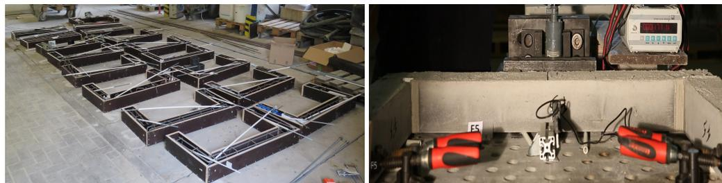
**Figure 1.** (Left) Preparation of the tested frames and (Right) testing setup (top beam: 1 m, sides: 0.5 m), recorded with two high-speed cameras.
