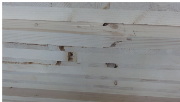
Figure 13. Failure of the 5-layer CLT panel after the experimental testing (detail).
