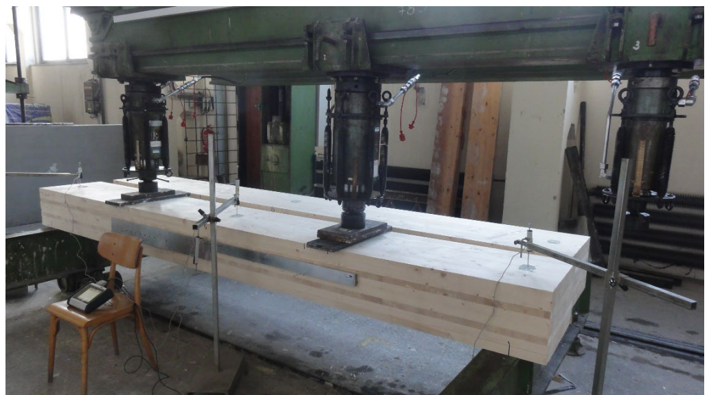
Figure 5. Test arrangement and positions of LVDTs.
