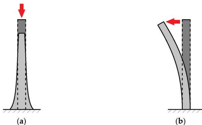
**Figure 1.** Wall failure by (a) plastic collapse and (b) elastic buckling [26].
