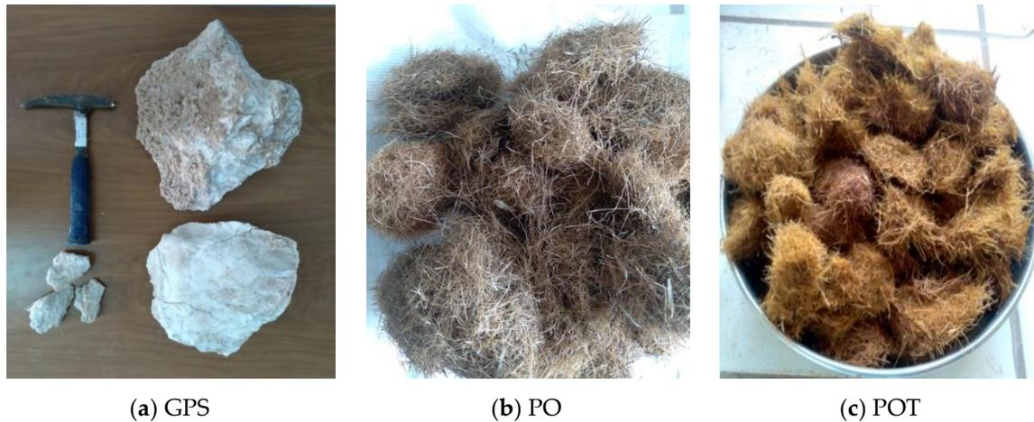
**Figure 1.** (a) The slices of gypsum (GPS), (b) Posidonia oceanica fibers (PO), and (c) the treated Posidonia oceanica fibers (POT).
