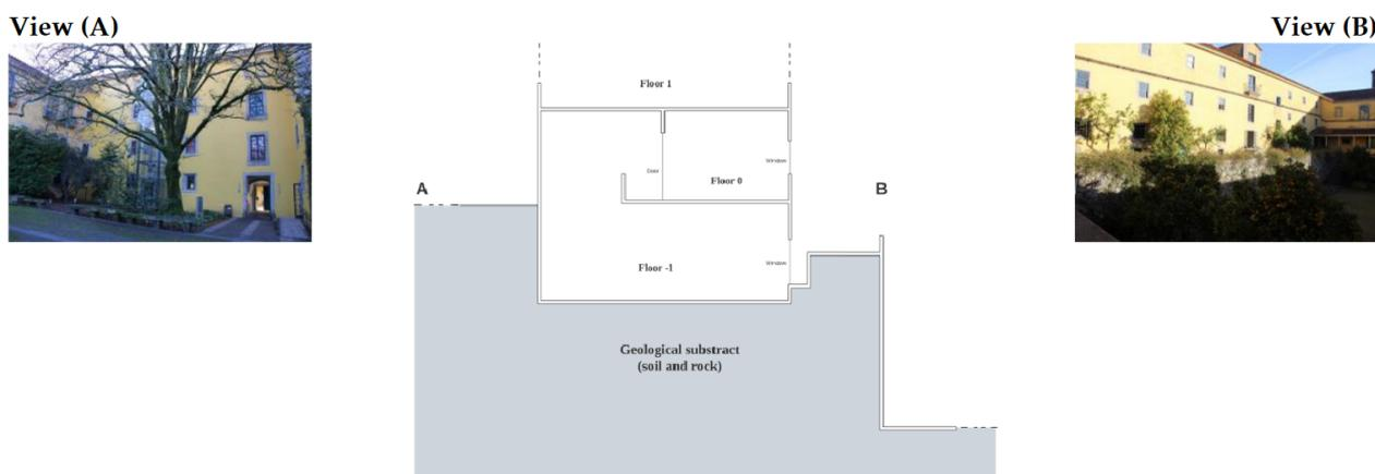
**Figure 2.** Section of the implantation of the building on the geological substratum. Views from each side of the main academic building of ESA IPVC, where view (A) refers to the main entrance of the building, exposed to the N, and view (B) presents the opposite facade, exposed to the S, where it is visible the difference of six meters between Floor -1 and the inner patio.
