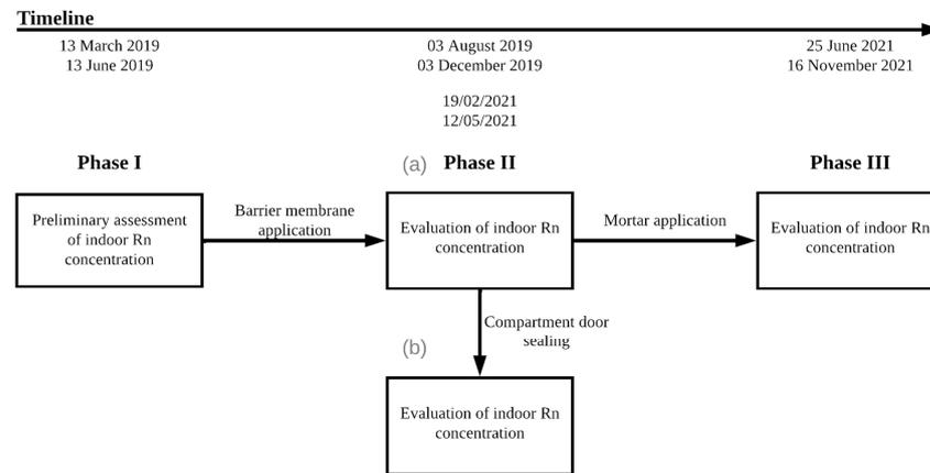
**Figure 3.** Organization of the works carried out during the monitoring process of the indoor Rn concentration in the compartment selected for the present case study.
