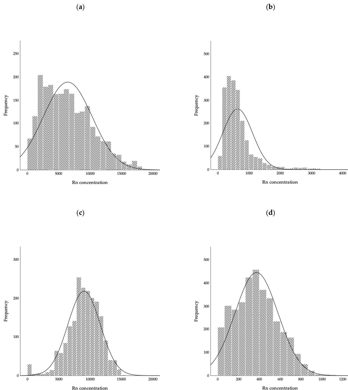
**Figure 9.** Histograms of the frequency distribution of occurrences. (a) Preliminary Phase I Assessment; (b) evaluation after application of the barrier membrane in Phase II(a); (c) evaluation after sealing the compartment door in Phase II(b); (d) evaluation after applying the coating mortar in Phase III.
