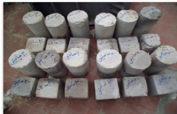
Figure 5. Shapes of specimens after heating.
