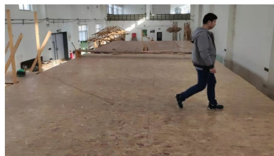
Figure 13. Pedestrian load test.
