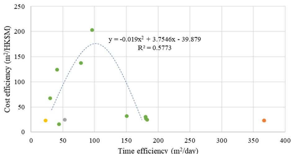
**Figure 7.** Measured time-efficiency and cost-efficiency. Notes: green dots—Projects A to I (modular QCs); yellow dot—Project J (conventional QC); orange dot—Project K (modular hospital); grey dot—Project L (conventional hospital).
