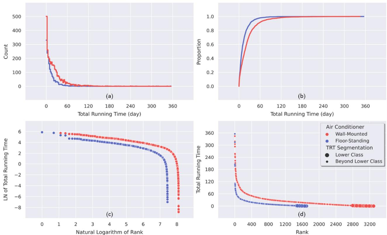
**Figure 4.** Lower Class segmentation of running time in bedroom and living-room cases. (a) histogram, (b) CDF, (c) log–log coordinate of rank-size and (d) Lower Class.
