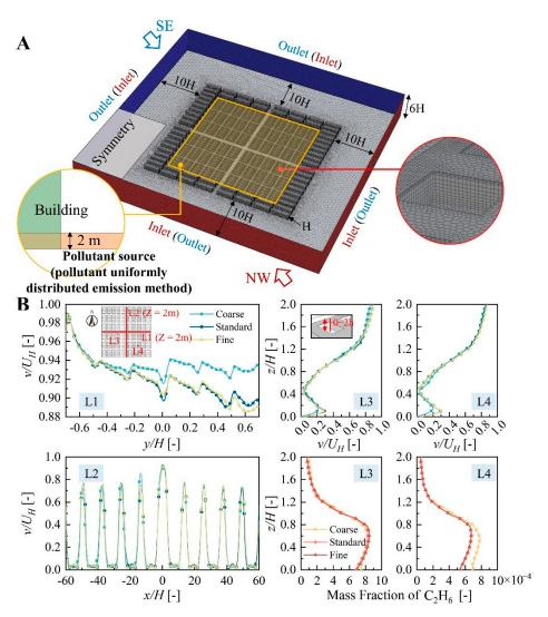
**Figure 5.** Computational domain and grid sensitivity analysis. (A) Computational domain dimensions and boundary condition settings. (B) Grid sensitivity verification.
