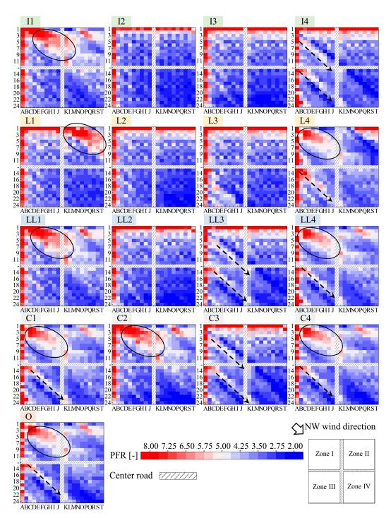
Figure 9. Analysis of the ventilation capacity of courtyards under northwest wind direction.
