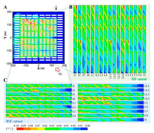
**Figure 8.** Contours of normalized pollutant concentration ( $C^*$ ) at the pedestrian level (Z = 1.5 m) for southeast wind direction. (**A**) Morphology O. (**B**) NS street of different morphology. (**C**) WE street of different morphology.
