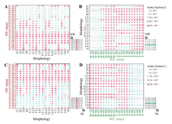
**Figure 14.** Intake fraction of the different zone in the central street. (**A**) and (**B**) under northwest wind direction (NW). (**C**) and (**D**) under southeast wind direction (SE). The red circles are intake fractions greater than  $12 \times 10^{-8}$ , and the green and blue circles are intake fractions less than  $12 \times 10^{-8}$ .  $12 \times 10^{-8}$  is the average value of intake fraction for all street zones.
