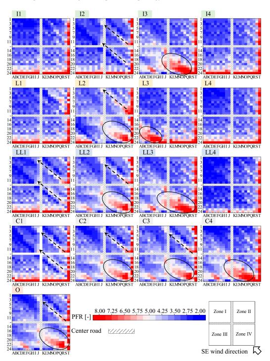
Figure 10. Analysis of the ventilation capacity of courtyards under southeast wind direction.
