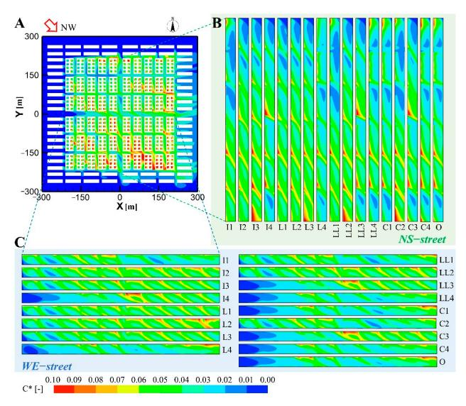
**Figure 7.** Contours of normalized pollutant concentration ( $C^*$ ) at the pedestrian level (Z = 1.5 m) for northwest wind direction. (**A**) Morphology O. (**B**) NS street of different morphology. (**C**) WE street of different morphology.
