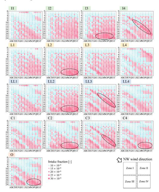
**Figure 12.** Analysis of the intake fraction of courtyards in the northwest wind direction. The red circles are intake fractions greater than  $15 \times 10^{-8}$ , and the blue circles are intake fractions less than  $15 \times 10^{-8}$ .  $15 \times 10^{-8}$  is the average value of intake fraction for all courtyards.
