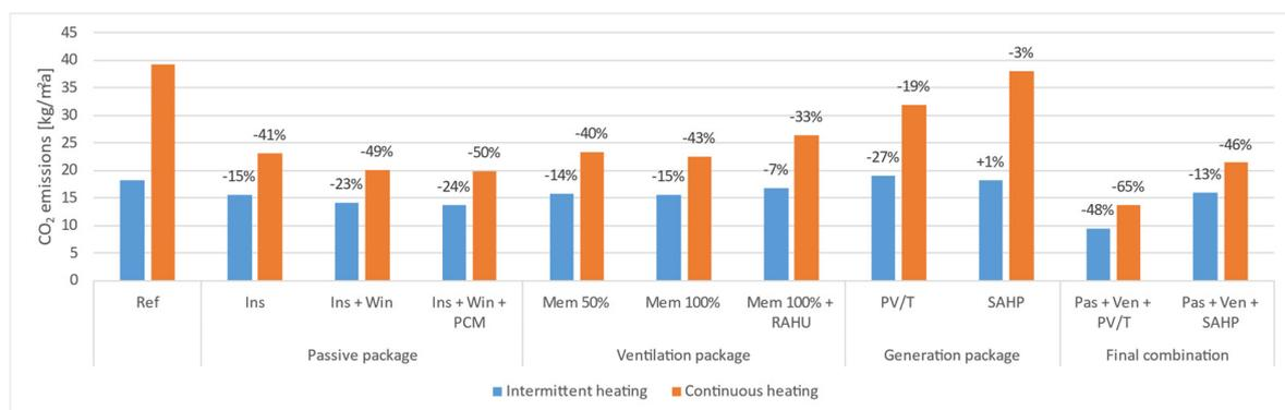
**Figure 7.** Intermittent heating vs. continuous heating: simulated relative CO<sub>2</sub> emissions reductions after renovating the Greek demo building.
