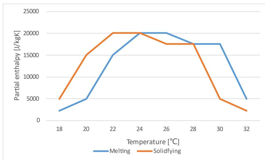
**Figure 5.** Melting and solidifying curves of the PCM product S21.
