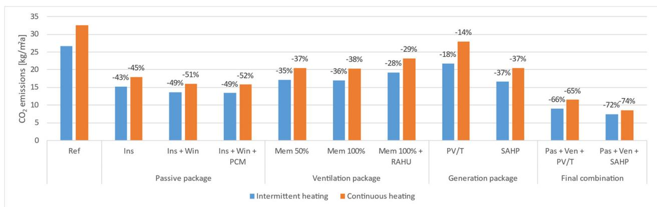
**Figure 11.** Intermittent heating vs. continuous heating: simulated relative CO<sub>2</sub> emissions reductions after renovating the Spanish demo building.
