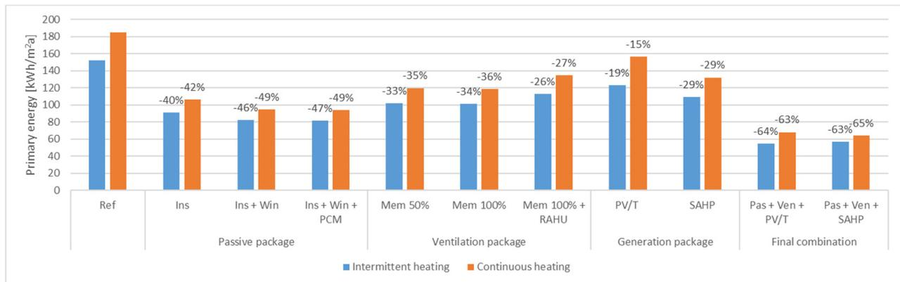
**Figure 10.** Intermittent heating vs. continuous heating: simulated relative primary energy reductions after renovating the Spanish demo building.
