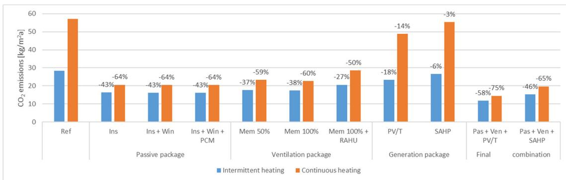
**Figure 9.** Intermittent heating vs. continuous heating: simulated relative CO<sub>2</sub> emissions reductions after renovating the Portuguese demo building.
