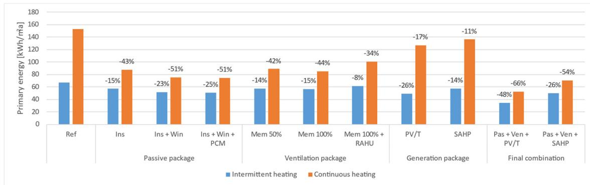
**Figure 6.** Intermittent heating vs. continuous heating: simulated relative primary energy reductions after renovating the Greek demo building.
