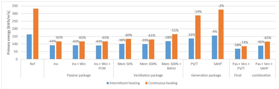
**Figure 8.** Intermittent heating vs. continuous heating: simulated relative primary energy reductions after renovating the Portuguese demo building.
