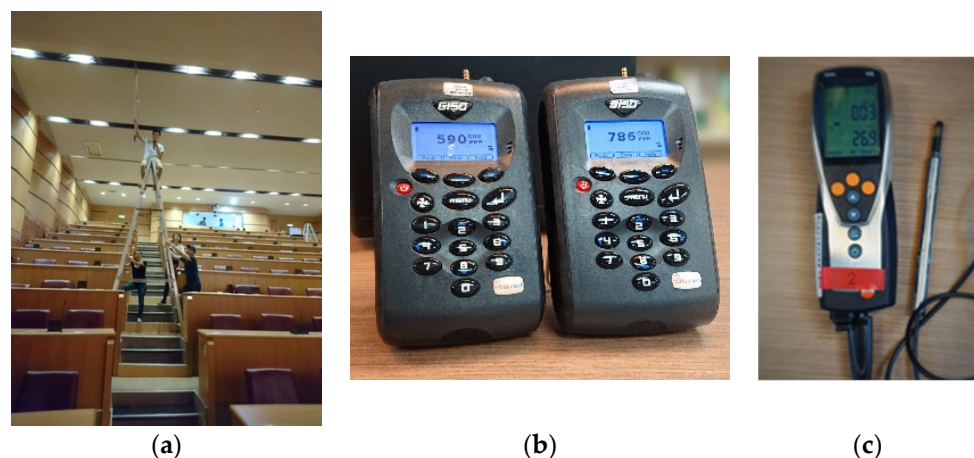
Figure 2. Actual measurement in the field: (a) Air velocity measurement in the inlet; (b) Geotech G150 CO 2 sensor; (c) Anemometer TESTO 435-2.
