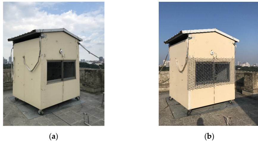
Figure 2. Photo of experimental house. (a) Without Expanded Metal Mesh; (b) With Expanded Metal Mesh.
