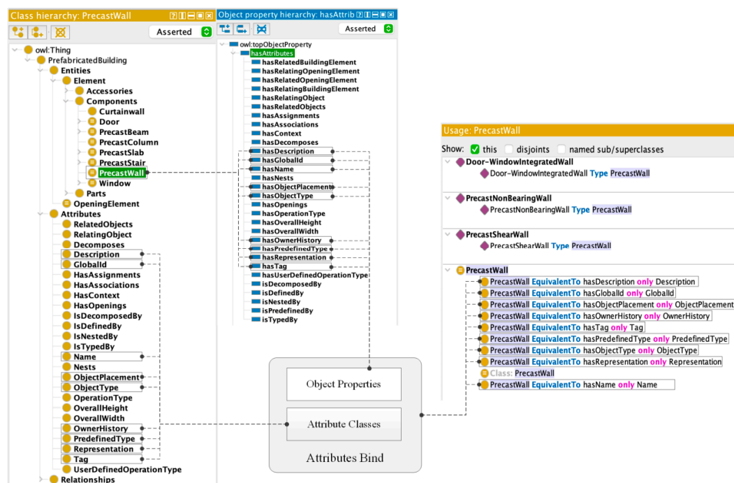
Figure 11. Relationship between prefabricated wall class and attribute classes through object properties.
