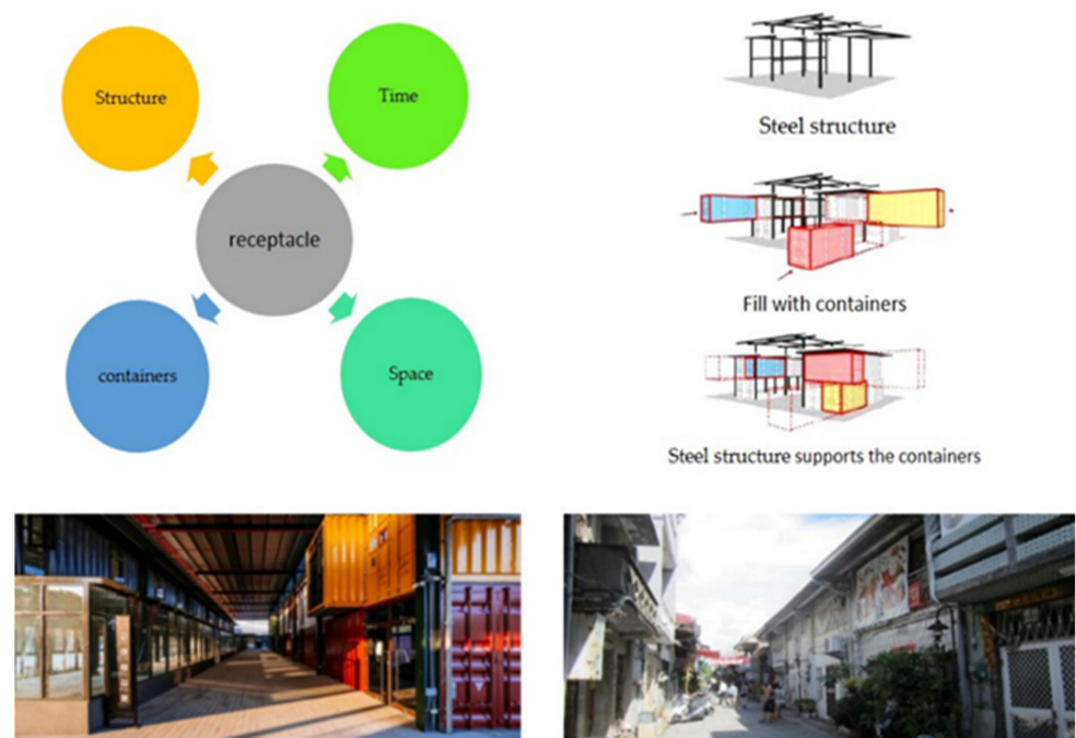
Figure 14. Diagram of the design concept, for fusing public art and architectural engineering. (Upper right structure diagram: Committee of public art installation project on Tainan Bus Station) [21].
