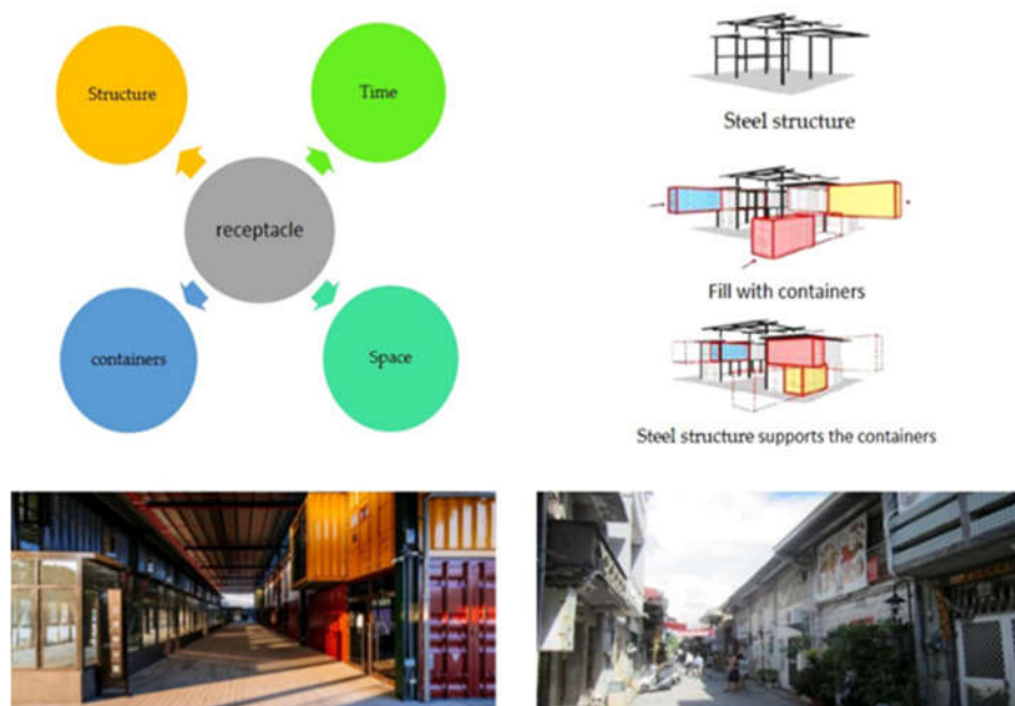
Figure 14. Diagram of the design concept, for fusing public art and architectural engineering. (Upper right structure diagram: Committee of public art installation project on Tainan Bus Station) [21].
