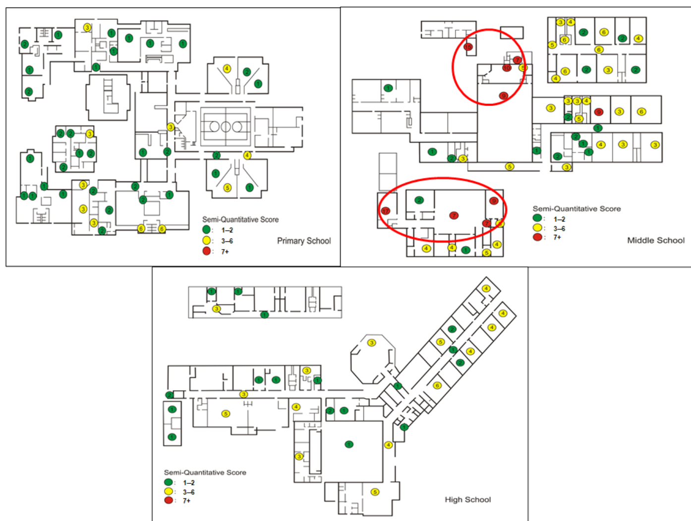
Figure 7. School floor maps showing the dampness and mold scores, color coded by the level of damage, with green = low, yellow = medium, and red = high. This identifies the most water-damaged areas within the school buildings.
