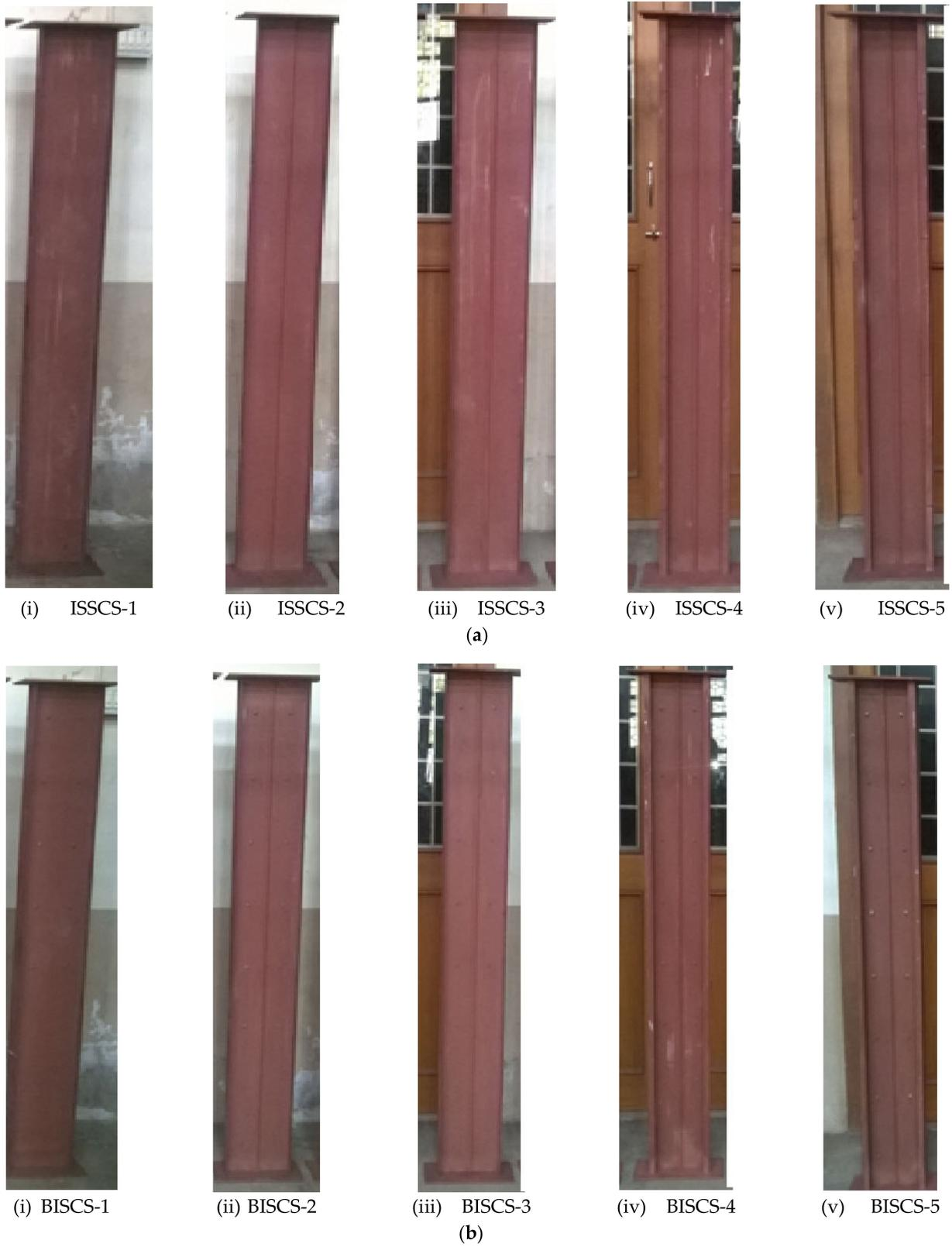
**Figure 7.** Specimens for experimentation. (a) Single Sections. (b) Double sections.
