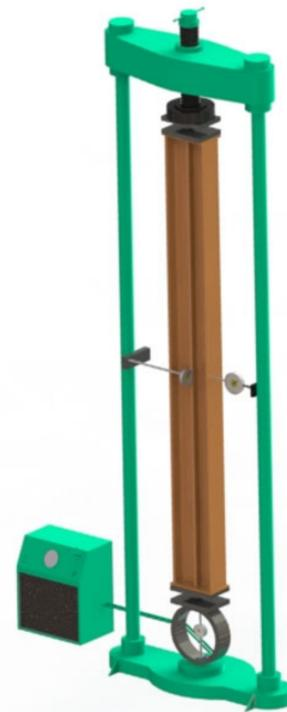
(b) Graphical drawing of the test rig-Long column
