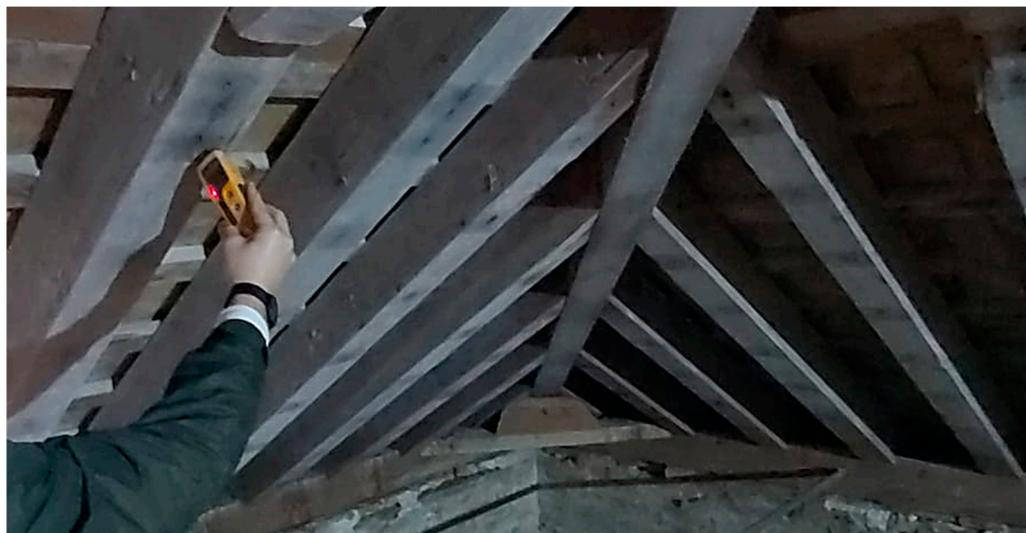
**Figure 11.** Protimeter Survemaster SM measuring the wood moisture content.
