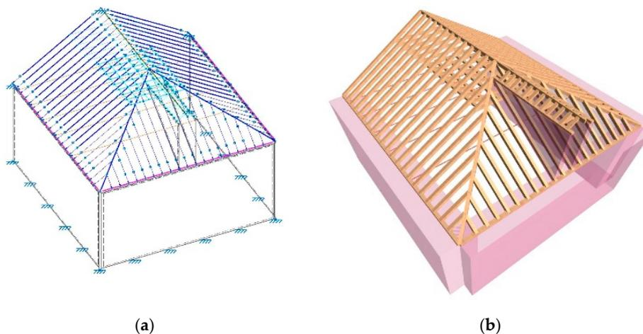
**Figure 18.** Structure models: (a) structure modelled in CYPE software; (b) realistic representation of the CYPE model.
