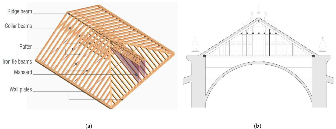
**Figure 6.** (a) Structural diagram and glossary of specific timber terms; (b) section on the roof and the timber frame over the brick vault.
