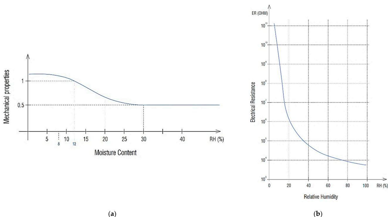
**Figure 10.** (a) Relationship between moisture content and mechanical properties of the timber [24]; (b) relationship between RH and electrical resistance [22].
