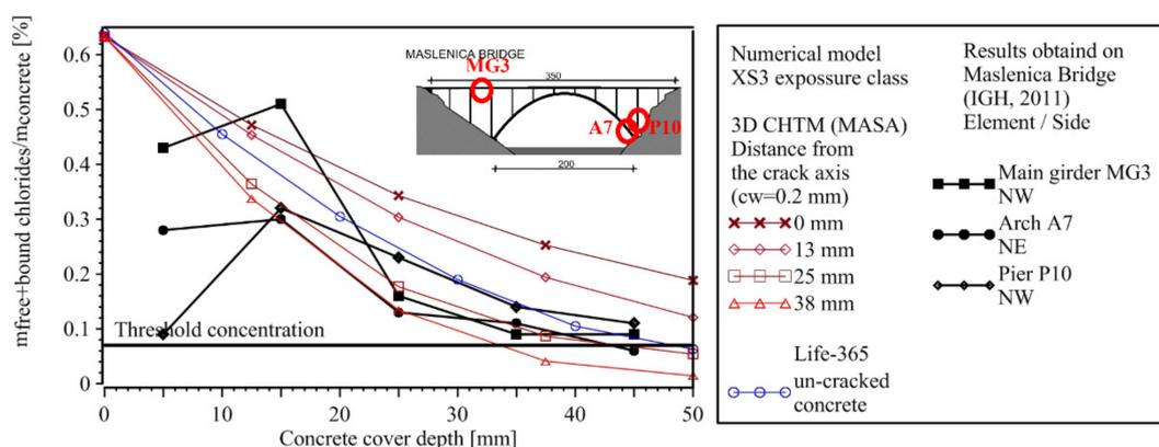
**Figure 6.** The total chloride content in concrete after 13 years of sea exposure: comparison of the numerical results and measured values on the Maslenica Bridge (reproduced with permission from [40], IOP Proceedings, 2019).
