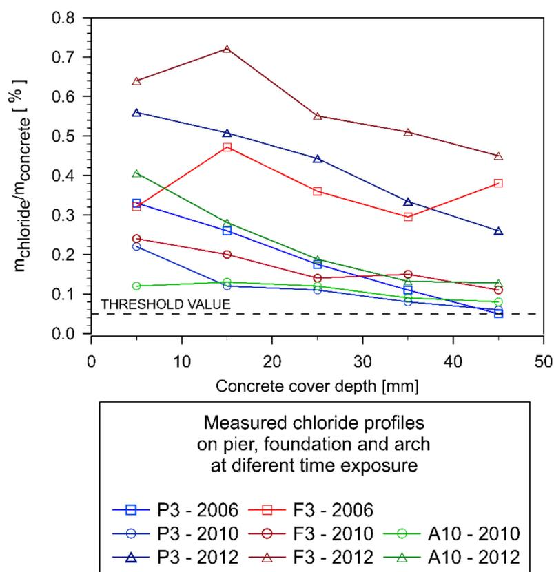
**Figure 5.** Measured chloride profile on pier P3 (15 m above sea level, surface exposed to NNE), joint pier P3 and arch foundation F3 (10 m above sea level, surface exposed to ENE), and arch segment close to the arch foundation at pier P10 (10 m above sea level, surface exposed to ENE) in different time periods: 2006, 2010 and 2012.
