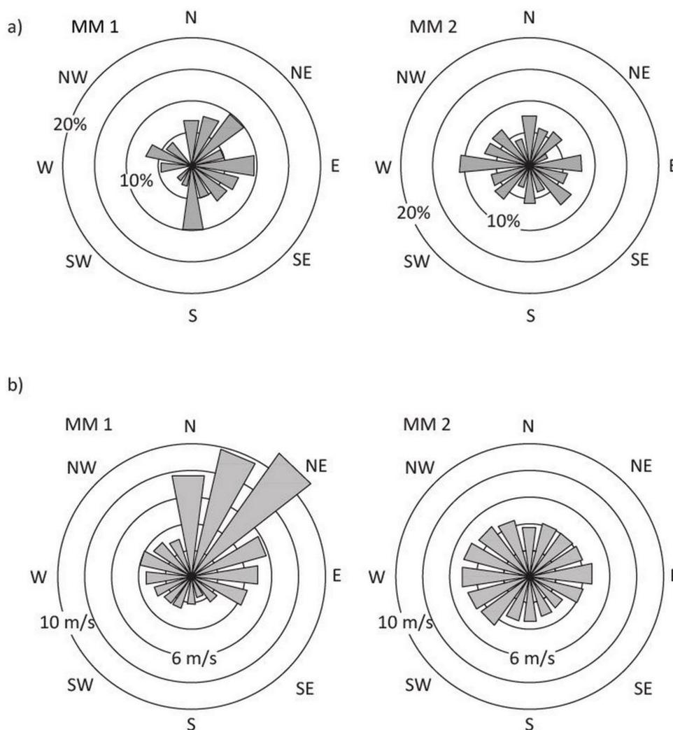
**Figure 7.** Distribution of (a) frequencies and (b) medium speed of wind direction at the observed meteorological stations for the periods 1998–2002 (for MM1) and 2000–2002 (for MM2) (adapted with permission from [43], Croatian Association of Civil Engineers, 2003).
