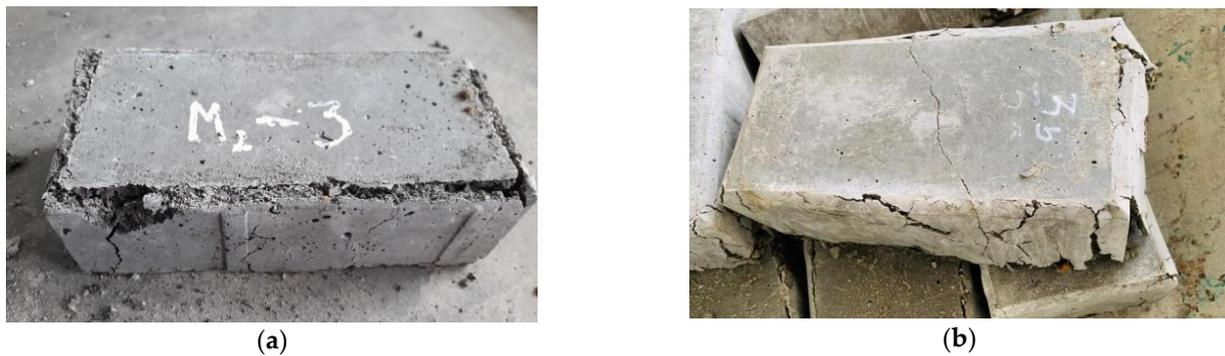
**Figure 7.** Failure Patterns of the IPB from Batch 1 and 2: (a) CR-based block; (b) CCF-based block.
